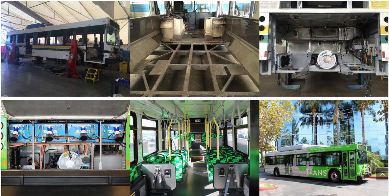
Figure 1-10 Complete Coach Works' process for repowering conventional buses to battery electric buses 211
