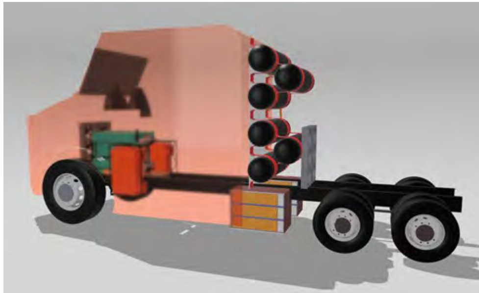
Figure 2 FEV High-Level FCEV Packaging Concept 395
