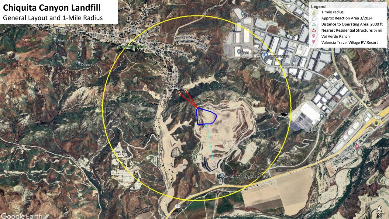
The reaction area and the working face of the landfill are 2,000 feet apart.
