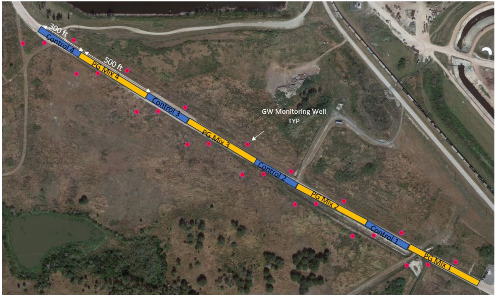
Figure 9-1: Groundwater monitoring well locations for each road base subsection
