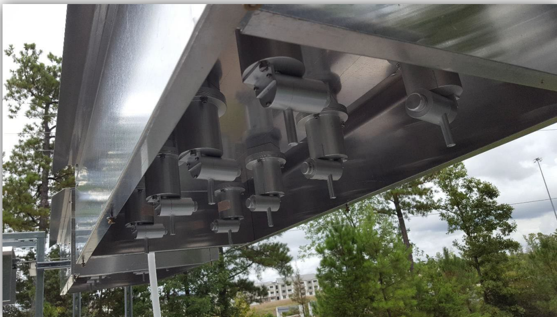
Figure 2. PE Sampling system consisting of 32 PM2.5 cyclones on four sampling manifolds and one dedicated pump (pump-box in the foreground):
