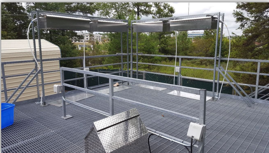
Figure 2. PE Sampling system consisting of 32 PM2.5 cyclones on four sampling manifolds and one dedicated pump (pump-box in the foreground):
