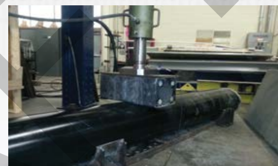
Crush Test on Concrete Filled Pile
