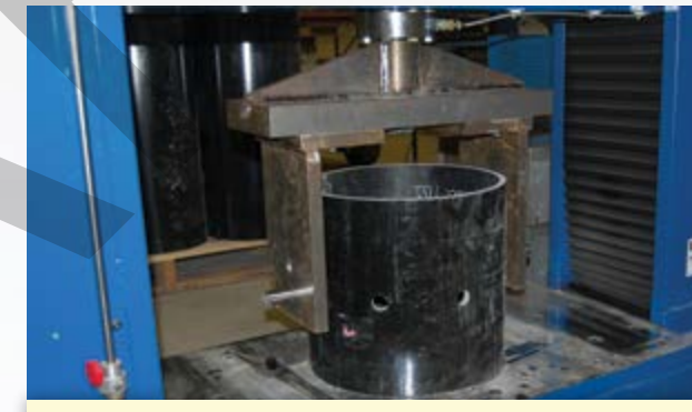
Bolted Connection Test - Parallel
