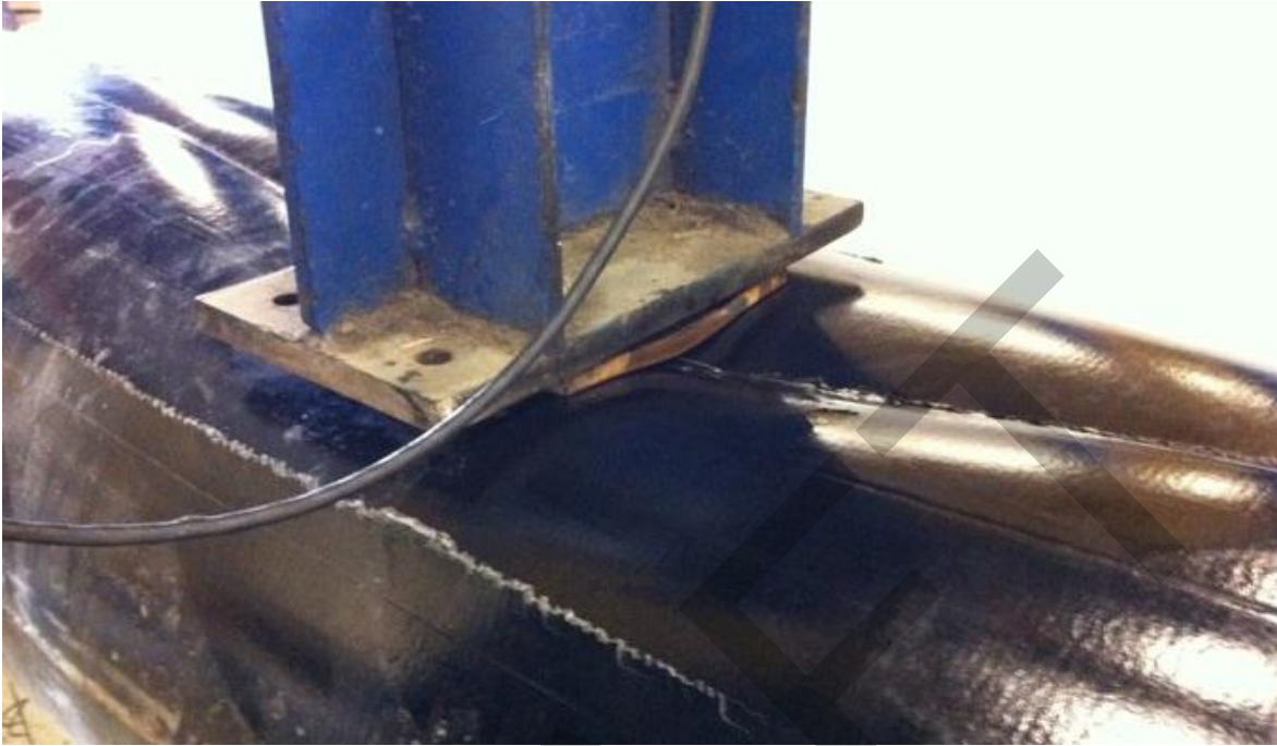
Figure 21: 16-in Sample with 6-in Washer at about 21 kips
