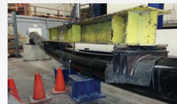
Full Section Testing of Concrete Filled Pile
