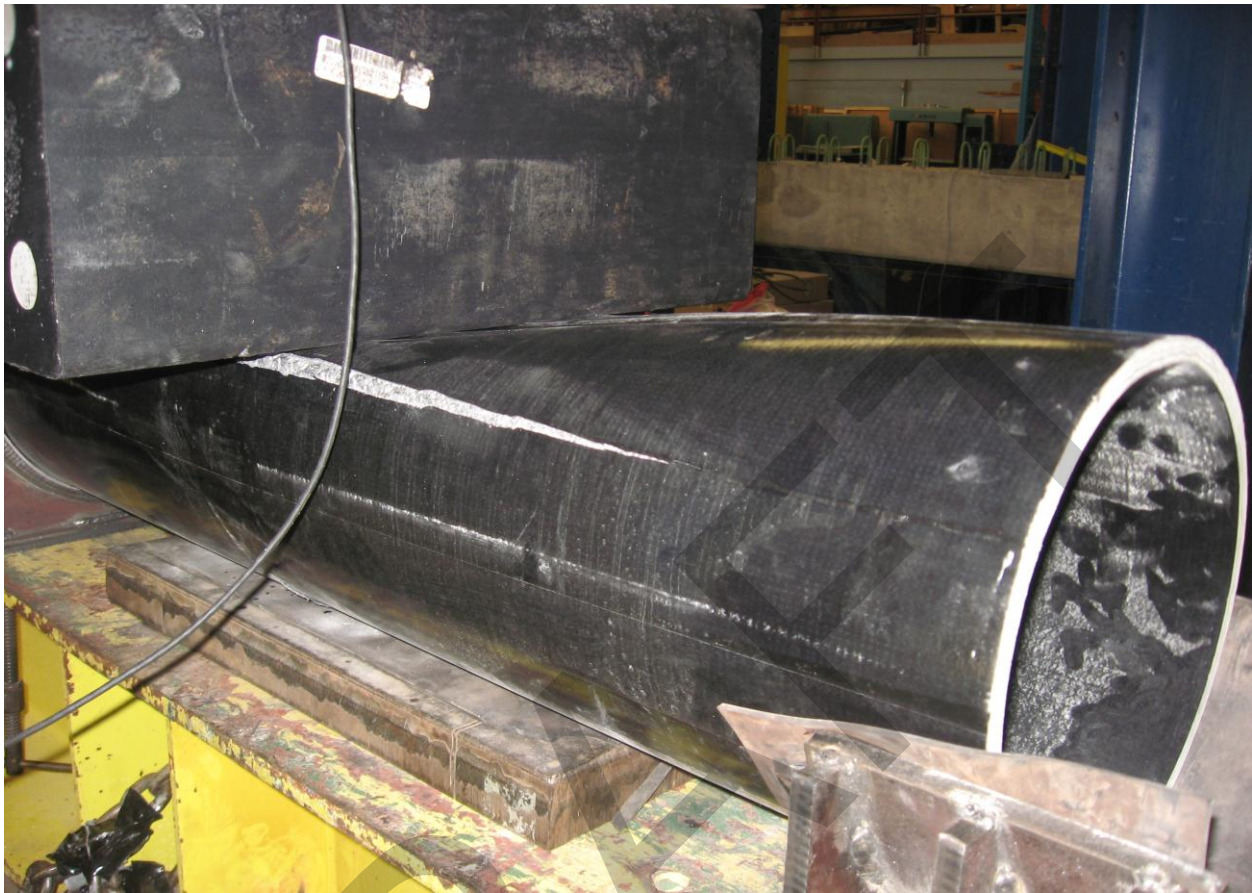
Figure 10: 12-inch Crush Test Pile Failure
