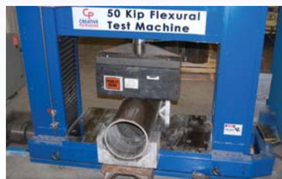
SUPERPILE® Crush Strength Test Set Up
