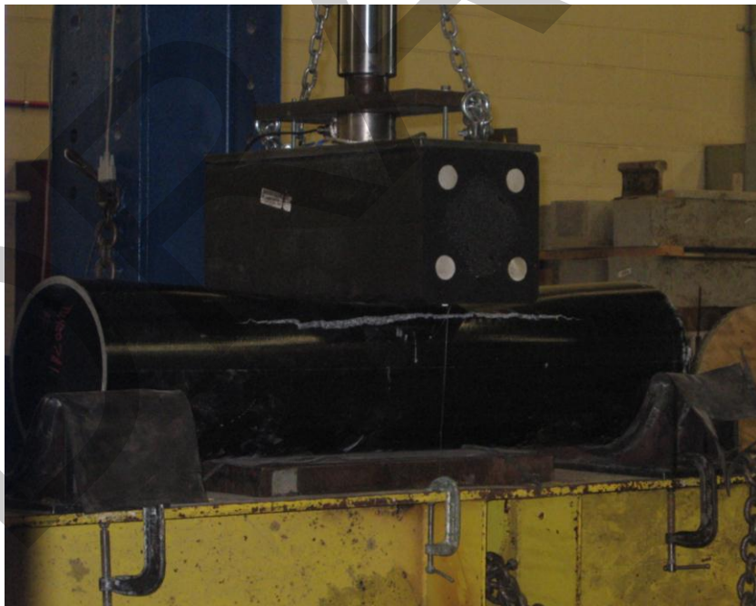
Figure 3: Crush Test: 12-inch pile
