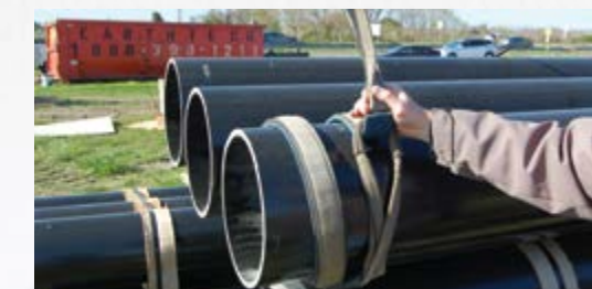
Lift-It® Sling Double Wrapped Around SUPERPILE®
