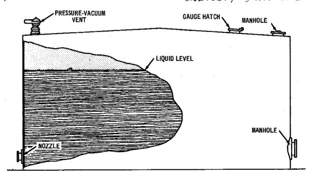
Figure 4.3-1. Fixed roof storage tank.
