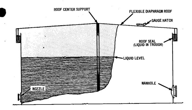
Figure 4.3-3. Variable vapor storage tank (wet-seal lifter type).
