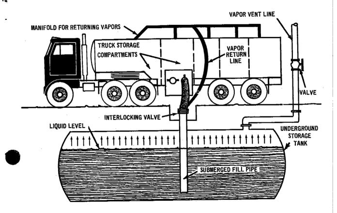
Figure 4.4-2. Underground storage tank vapor-recovery system1.
