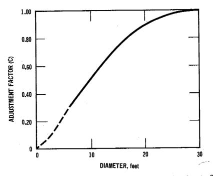
Figure 4.3-4. Adjustment factor for small-diameter fixed roof tanks.2
