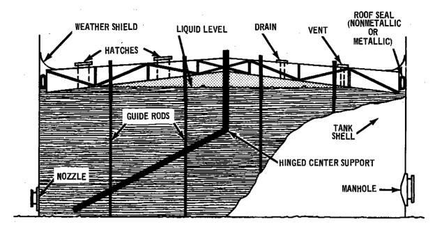
Figure 4.3-2. Double-deck floating roof storage tank (nonmetallic seal).
