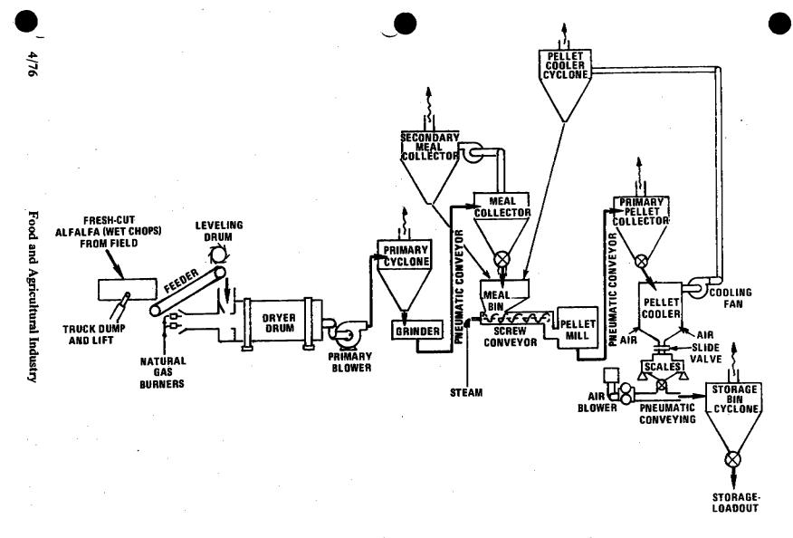
Figure 6.1-1. Generalized flow diagram for alfalfa dehydration plant.
