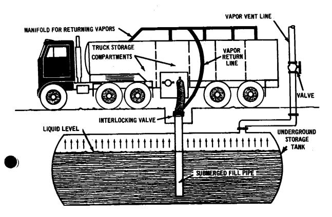
Figure 4.4-2. Underground storage tank vapor-recovery system1.
