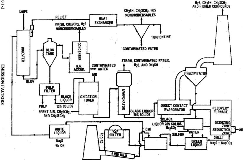
Figure 10.1.2-1. Typical kraft sulfate pulping and recovery process.
