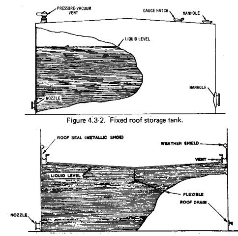
Figure 4.3-3. Pan-type floating roof storage tank (metallic seals).
