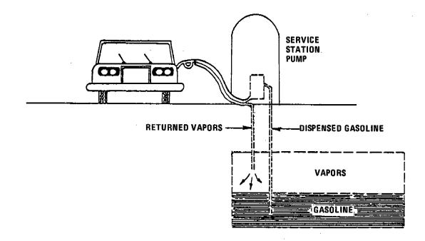
Figure 4.4-7. Automobile refueling vapor-recovery system.
