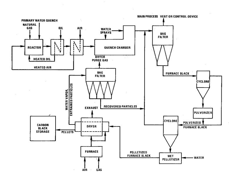
Figure 5.3-1. Simplified flow diagram of carbon black production by the oil-fired furnace process.
