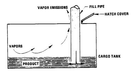
Figure 4.4-3. Submerged fill pipe.
