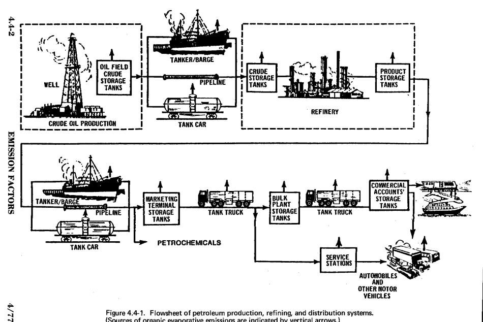
Figure 4.4-1. Flowsheet of petroleum production, refining, and distribution systems. (Sources of organic evaporative emissions are indicated by vertical arrows.)
