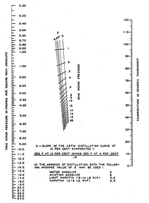
Figure 4.3-8. Vapor pressures of gasolines and finished petroleum products.
