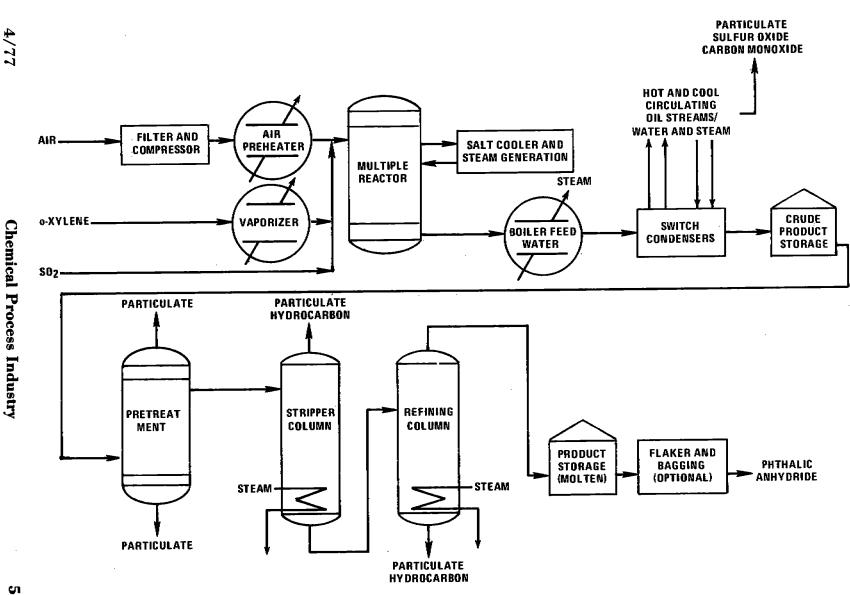
Figure 5.12-1. Flow diagram for phthalic anhydride using o-xylene as basic feedstock.<sup>1</sup>
