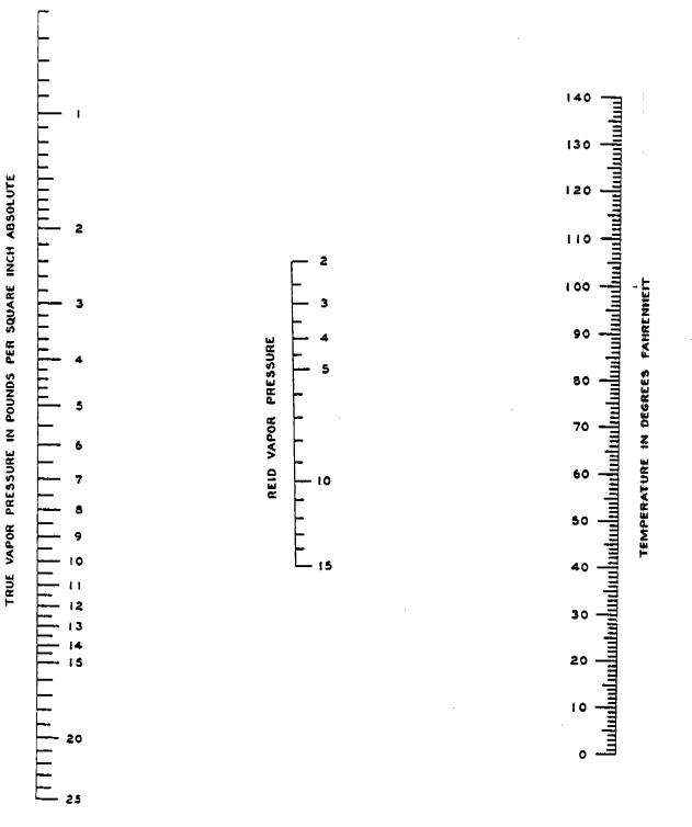
Figure 4.3-9. Vapor pressures of crude oil.
