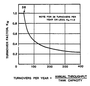
Figure 4.3-11. Turnover factor (K<sub>N</sub>) for fixed roof tanks.
