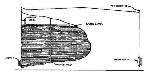
Figure 4.3-5. Covered floating roof storage tank.
