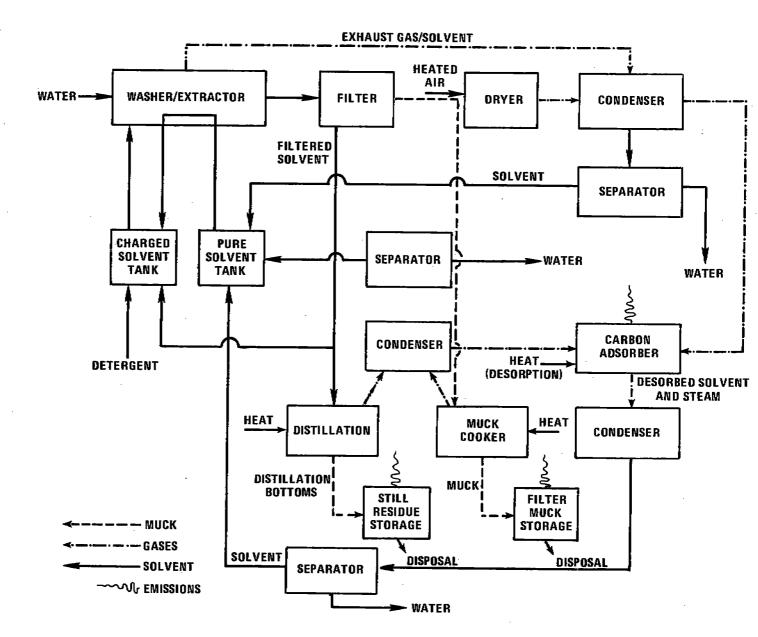
Figure 4.1-1. Perchloroethylene dry cleaning plant flow diagram.
