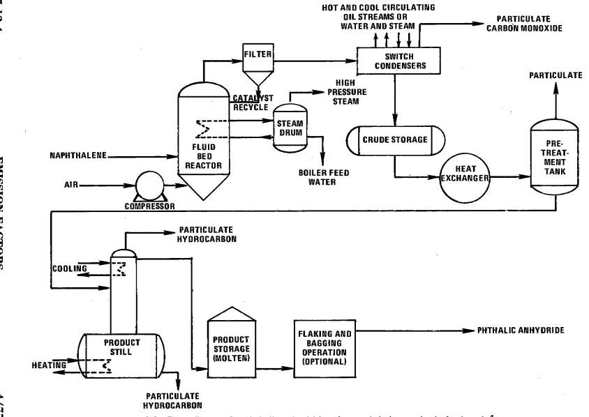
Figure 5.12-2. Flow diagram for phthalic anhydride using naphthalene as basic feedstock.1
