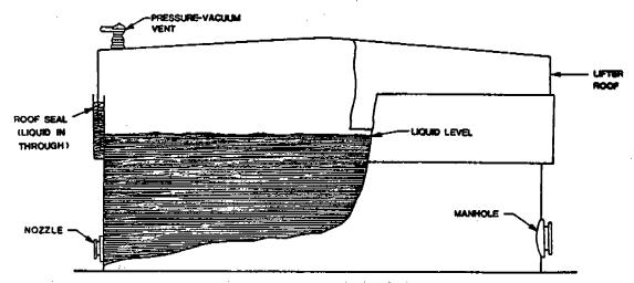
Figure 4.3-6. Lifter roof storage tank (wet seal).
