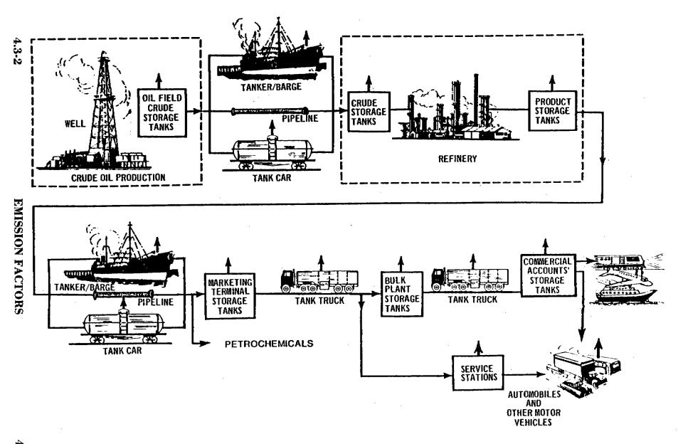
Figure 4.3-1. Flowsheet of petroleum production, refining, and distribution systems. (Sources of organic evaporative emissions are indicated by vertical arrows.)
