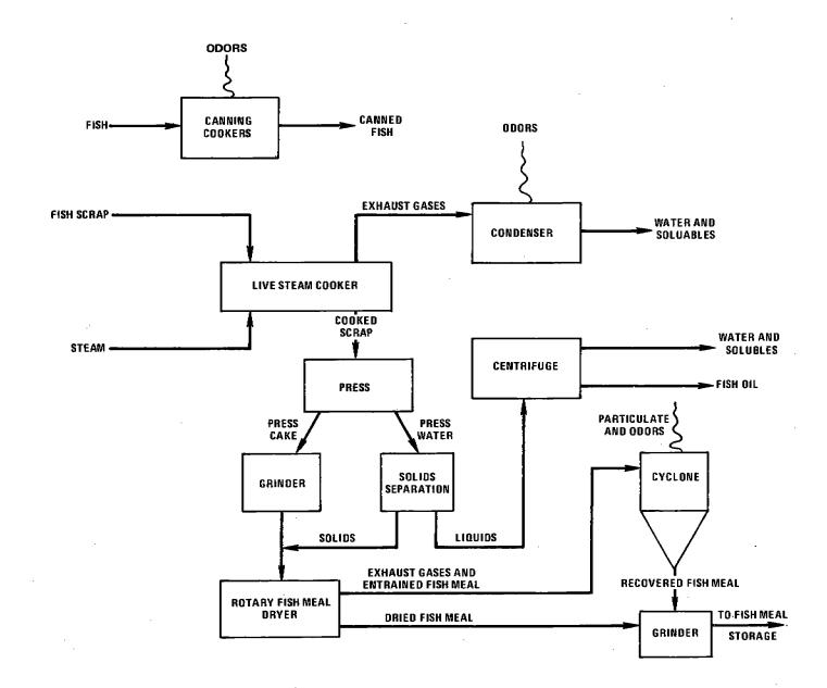
Figure 6.6-1. A generalized fish processing flow diagram.
