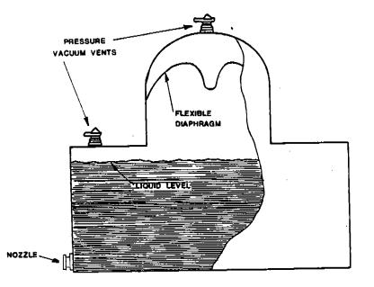
Figure 4.3-7. Flexible diaphragm tank (integral unit).
