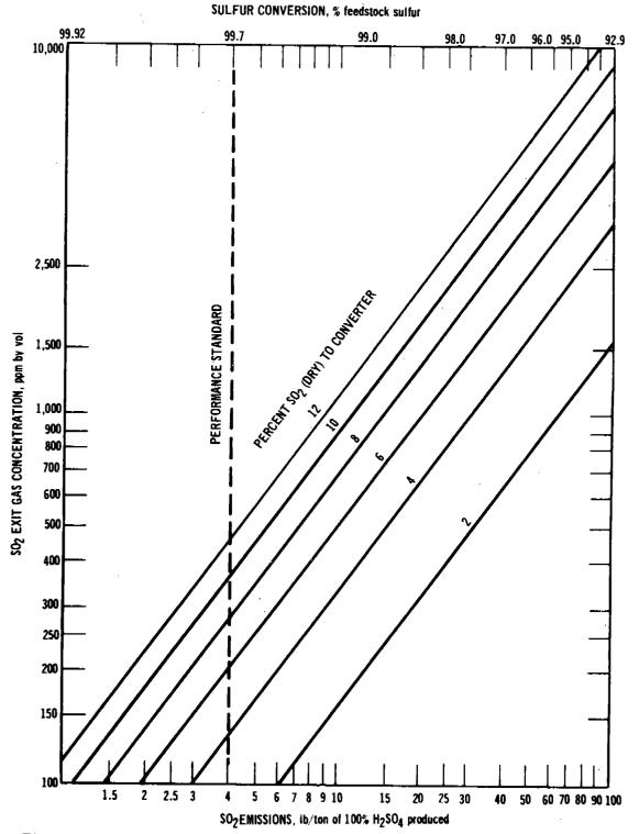
Figure 5.17-3. Sulfuric acid plant feedstock sulfur conversion versus volumetric and mass SO<sub>2</sub> emissions at various inlet SO<sub>2</sub> concentrations by volume.
