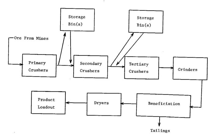
Figure 8.23-1. A metallic mineral processing plant.
