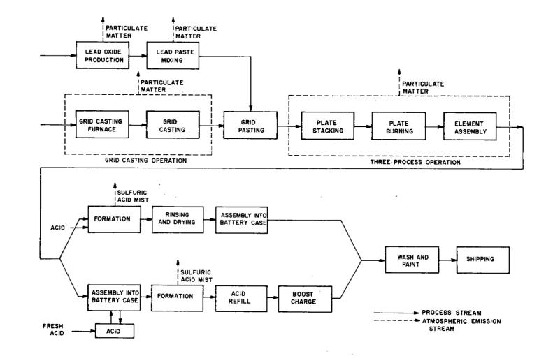
Figure 7.15-1. Process flow diagram for storage battery production.
