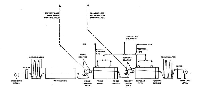
Figure 4.2.2.10-1. Flow Diagram of model coil coating line.
