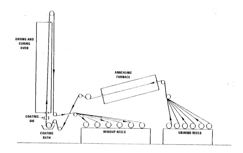
Figure 4.2.2.3-1. Wire coating line emission points.9
