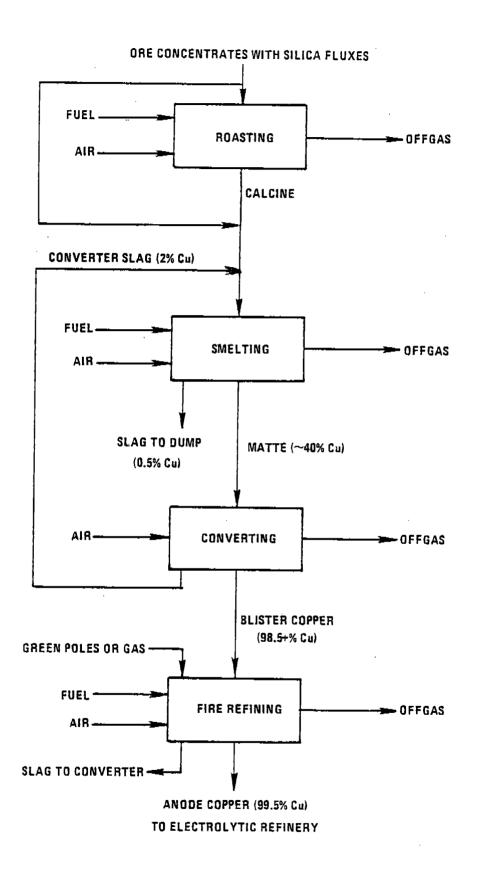
Figure 7.3-1. A conventional copper smelting process.
