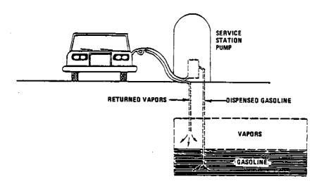
Figure 4.4-7. Automobile refueling vapor recovery system.
