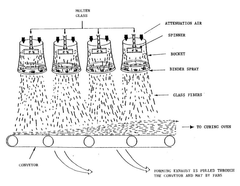
Figure 8.11-2. A typical rotary spin process.
