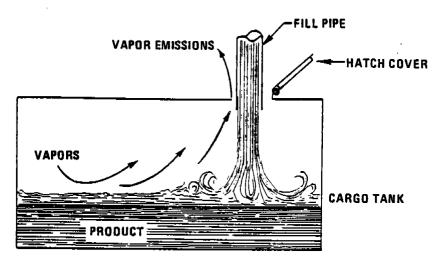
Figure 4.4-2. Splash loading method.
