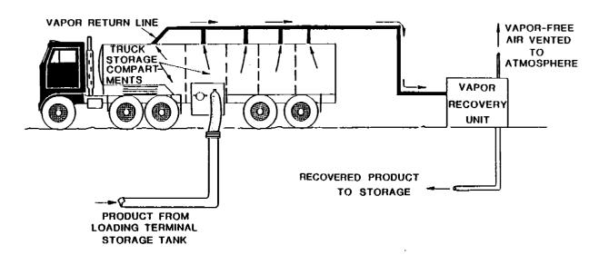
Figure 4.4-6. Tank truck loading with vapor recovery.
