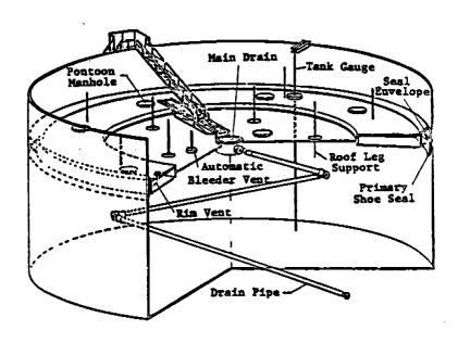
Figure 4.3-2. External floating roof tank. 1
