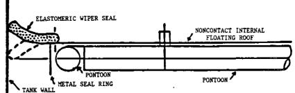
b. Elastomeric wiper seal.
