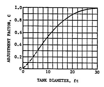
Figure 4.3-4. Adjustment factor (C) for small diameter tanks.  $^2$
