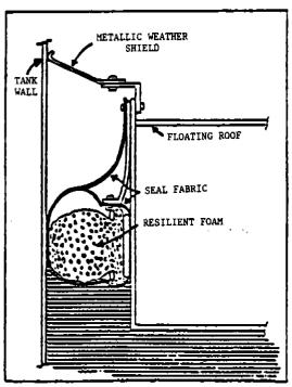
a. Liquid mounted seal with weather shield.
