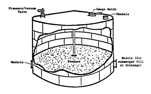
Figure 4.3-1. Typical fixed roof tank. 1
