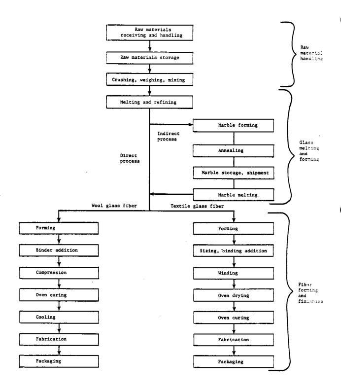
Figure 8.11-1. Typical flow diagram of the glass fiber production process.
