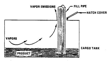
Figure 4.4-3. Submerged fill pipe.
