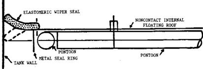
b. Elastomeric wiper seal.
