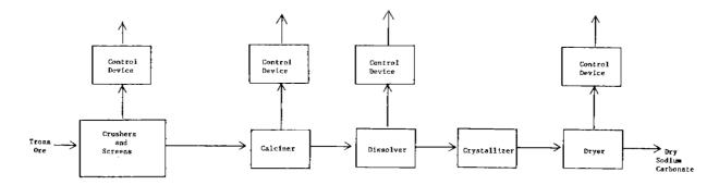
Figure 5.16-1. Sodium carbonate production by monohydrate process.
