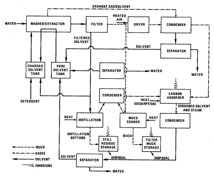
Figure 4.1-1. Perchloroethylene dry cleaning plant flow diagram.
