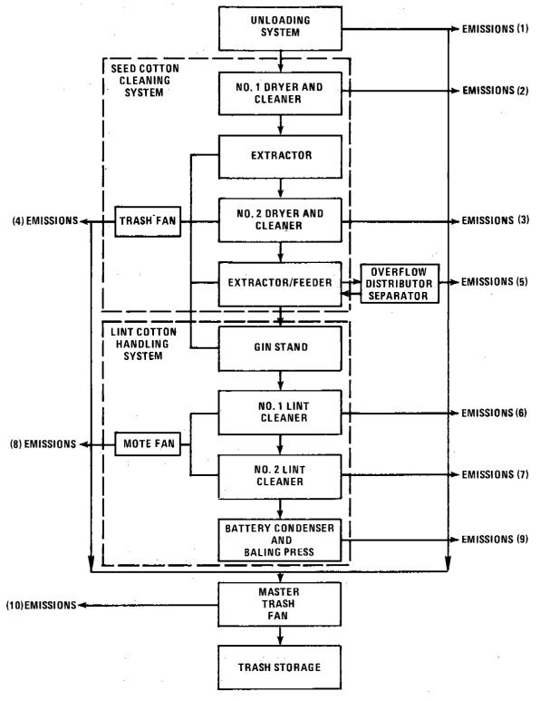
Figure 6.3-2. Emissions from a typical ginning operation.
