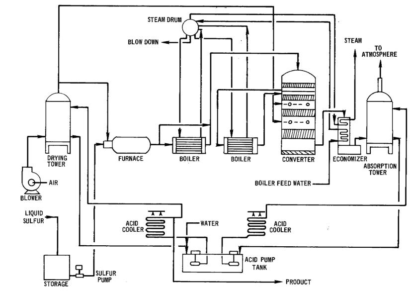
Figure 5.17-1. Basic flow diagram of contact process sulfuric acid plant burning elemental sulfur.
