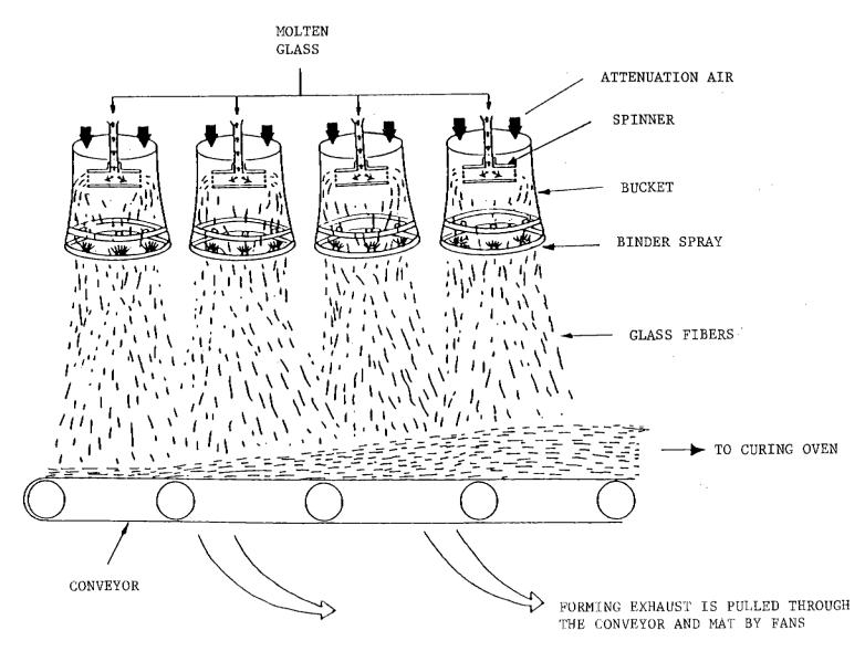
Figure 8.11-2. A typical rotary spin process.
