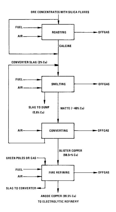
Figure 7.3-1. A conventional copper smelting process.
