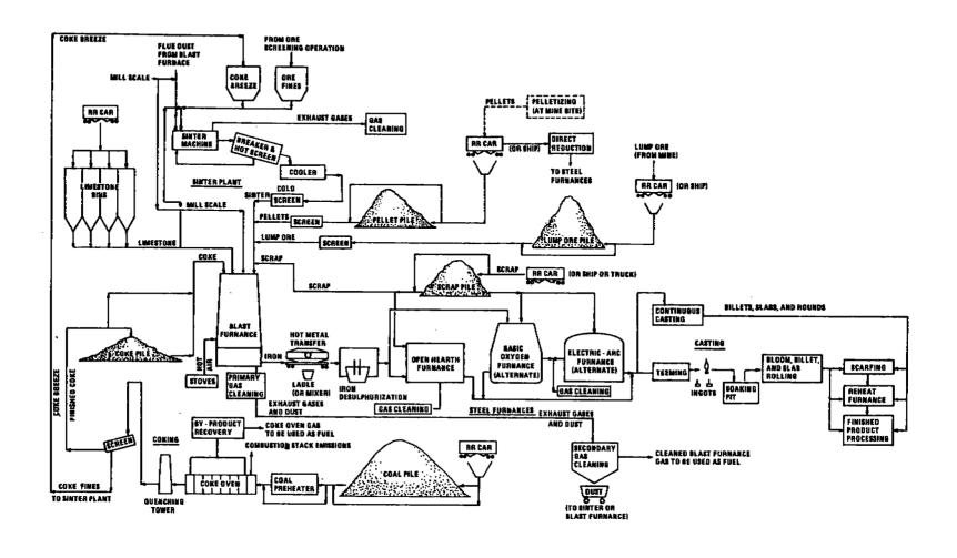
Figure 7.5-1. General flow diagram for the iron and steel industry.
