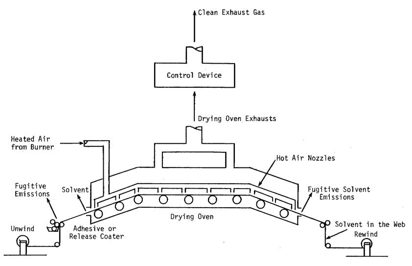
Figure 4.2.2.9-1. Diagram of a Pressure Sensitive Tape and Label Coating Line
