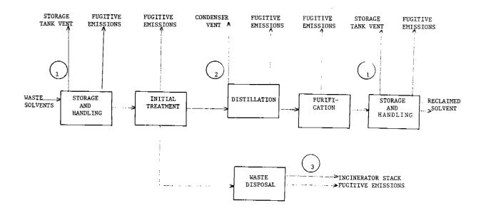
Figure 4.7-1. General waste solvent reclamation scheme and emission points. 1
