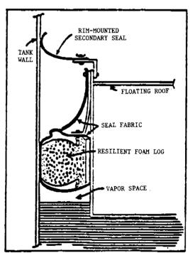
Vapor mounted seal with rim mounted secondary seal.
