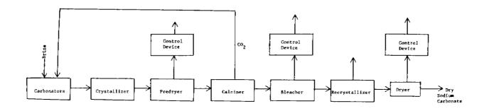
Figure 5.16-2. Sodium carbonate production by direct carbonation process.
