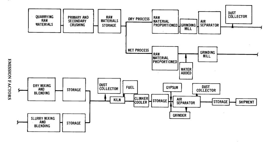
Figure 8.6-1. Basic flow diagram of portland cement manufacturing process.
