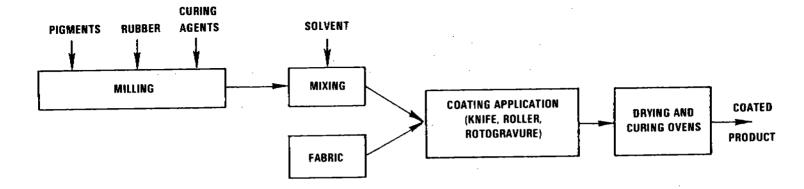
Figure 4.2.2.7-1. Fabric coating plant emission points.<sup>7</sup>
