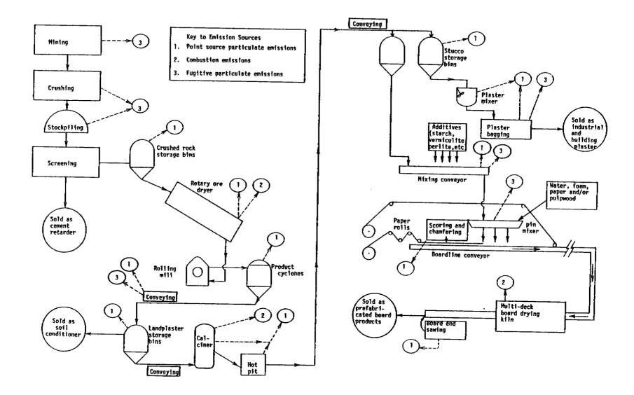
Figure 8.14-1. Overall gypsum manufacturing process flow diagram.
