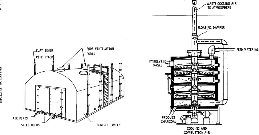
Figure 5.4-1. The Missouri type charcoal kiln (left) and the multiple hearth furnace (right).
