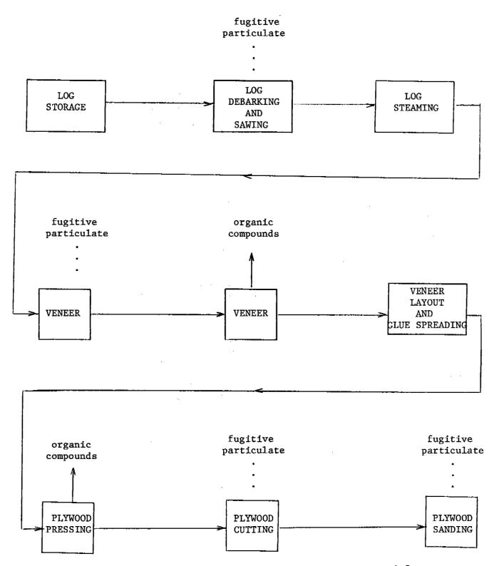
Figure 10.3-1. Plywood veneer and layout operations. $^{4,5}$
