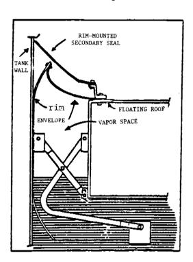
Metallic shoe seal with shoe mounted secondary seal.
