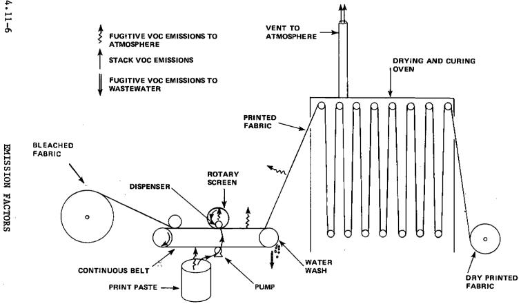
Figure 4.11-1. Schematic diagram of the rotary screen printing process, with fabric drying in a vented oven.
