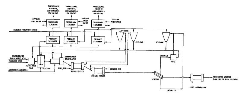
Figure 6.2.3-1. Ammonium phosphate process flow diagram.
