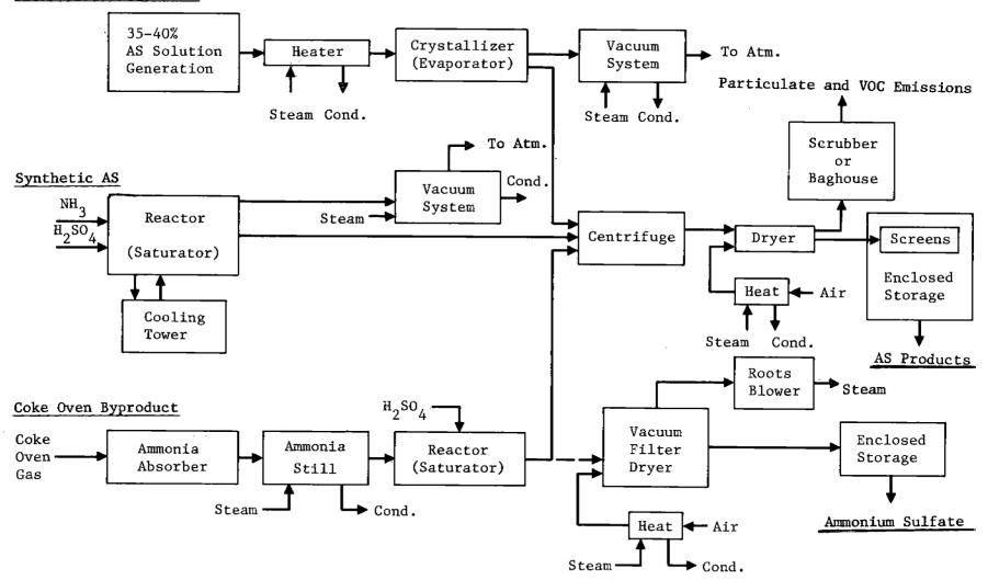
Figure 6.18-1. Diagram of Ammonium Sulfate (AS) processes.
