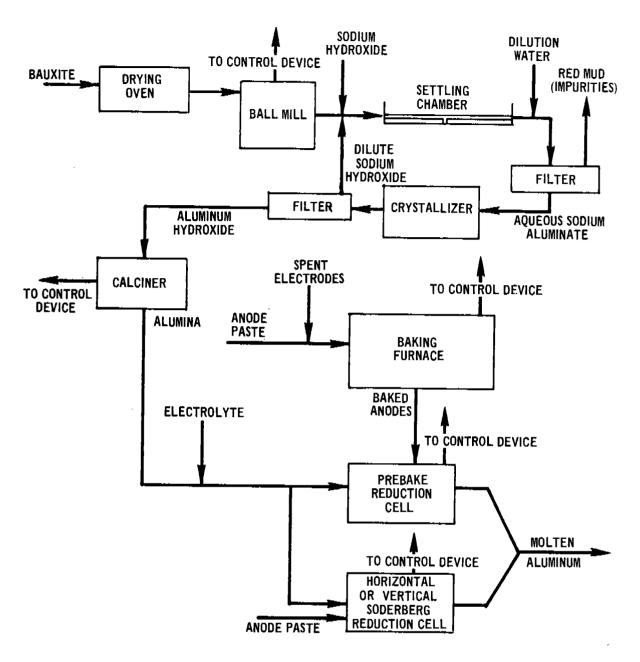
Figure 7.1-1. Schematic diagram of primary aluminum production process.
