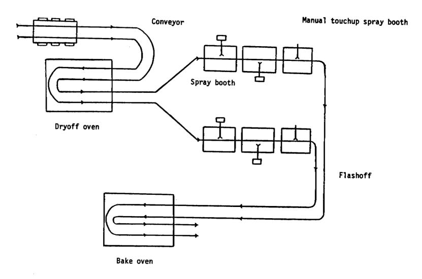
Figure 4.2.2.12-1. Example automated spray coating lines, with manual touchup.
