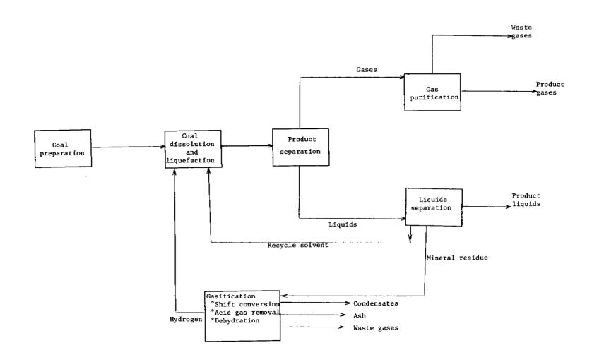
Figure 8.21-2. Flow diagram for an example coal liquefaction facility.
