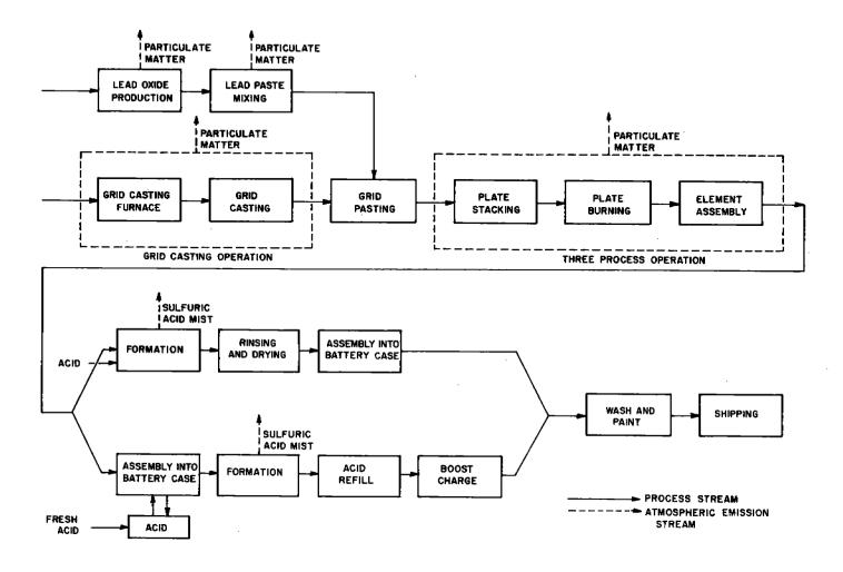
Figure 7.15-1. Process flow diagram for storage battery production.
