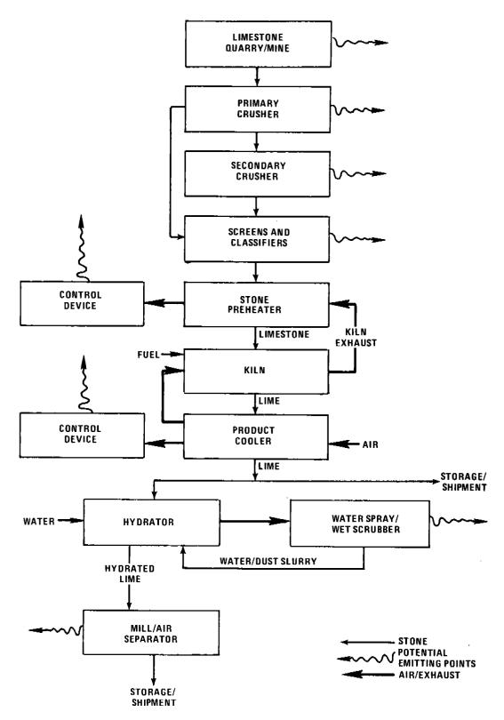
Figure 8.15-1. Generalized lime manufacturing plant.
