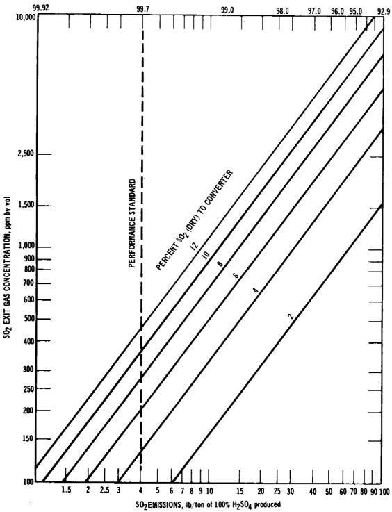
Figure 5.17-3. Sulfuric acid plant feedstock sulfur conversion versus volumetric and mass  $SO_2$  emissions at various inlet  $SO_2$  concentrations by volume.
