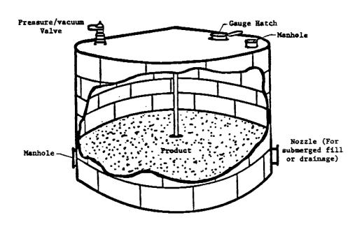
Figure 4.3-1. Typical fixed roof tank. 1
