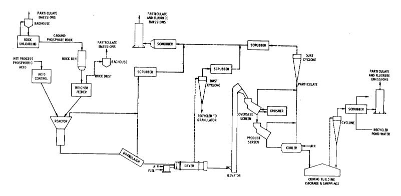
Figure 6.10.2-1. Dorr-Oliver process flow diagram for granular triple superphosphate production.
