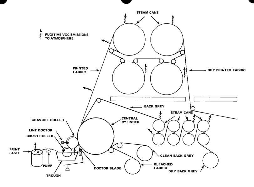
Figure 4.11-2. Schematic diagram of the roller printing process, with fabric drying on steam cans.
