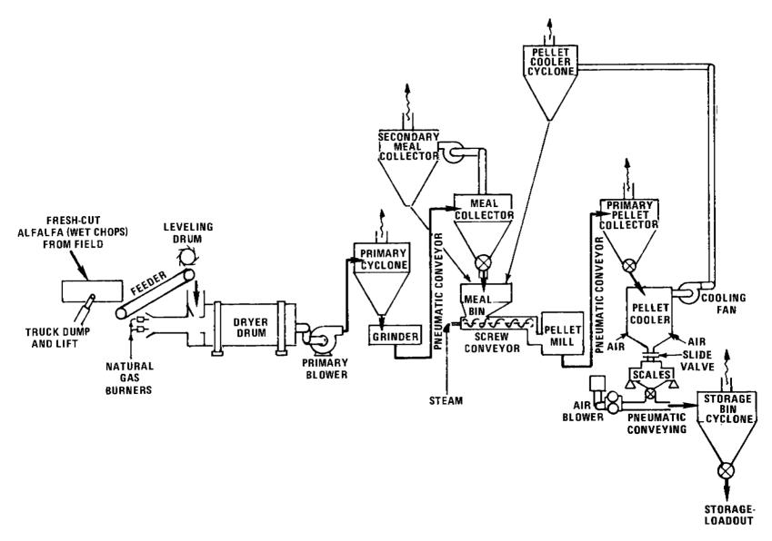
Figure 6.1-1. Generalized flow diagram for alfalfa dehydration plant.
