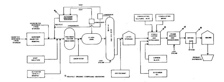
Figure 5.20-1. Typical process for crumb production by emulsion polymerization.
