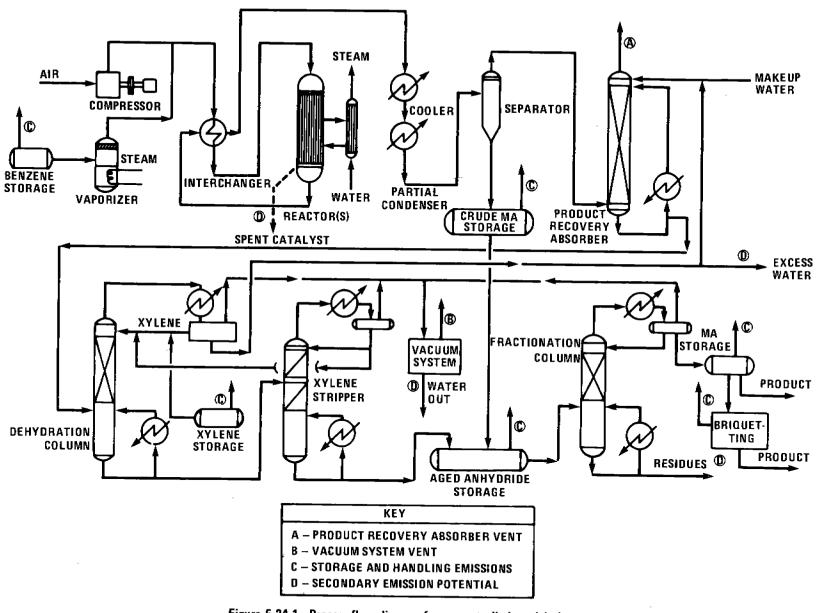
Figure 5.24-1. Process flow diagram for uncontrolled model plant.
