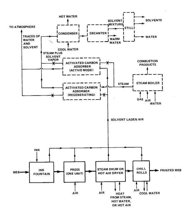
Figure 4.9-3. Rotogravure and flexography printing line emission points (chill rolls not used in rotogravure publication printing).<sup>11</sup>
