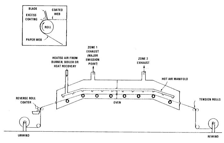
Figure 4.2.2.6.-1. Paper coating line emission points. 7
