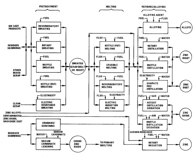
Figure 7.14-1. Process flow diagram of secondary zinc processing.
