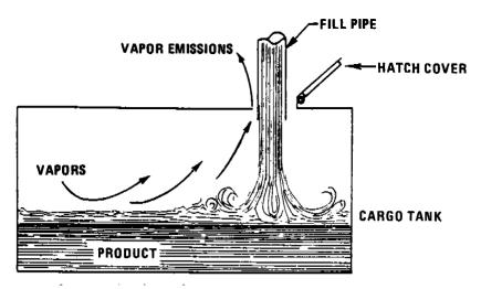
Figure 4.4-2. Splash loading method.
