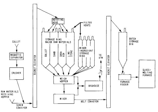
8.13-2. Flow diagram of a batch plant.1
