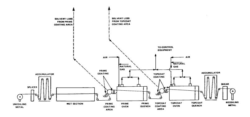
Figure 4.2.2.10-1. Flow Diagram of model coil coating line.
