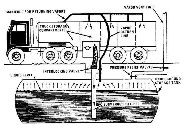
Figure 4.4-5. Tank truck unloading into a service station underground storage tank and practicing "vapor balance" form of emission control.
