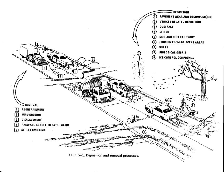
The total loading (excluding litter) is measured by sweeping and vacuuming lateral strips of known area from each active travel lane. The silt fraction is determined by measuring the proportion of loose dry road dust that passes a 200 mesh screen, using the ASTM-C-136 method. Silt loading is the product of total loading and silt content.
