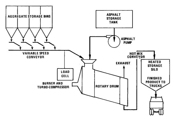
8.1-3. Shearer type dryer-drum hot asphalt plant.
