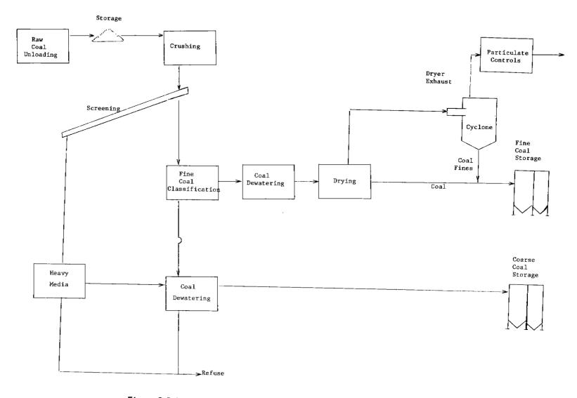
Figure 8.9-1. Typical coal cleaning plant process flow diagram.
