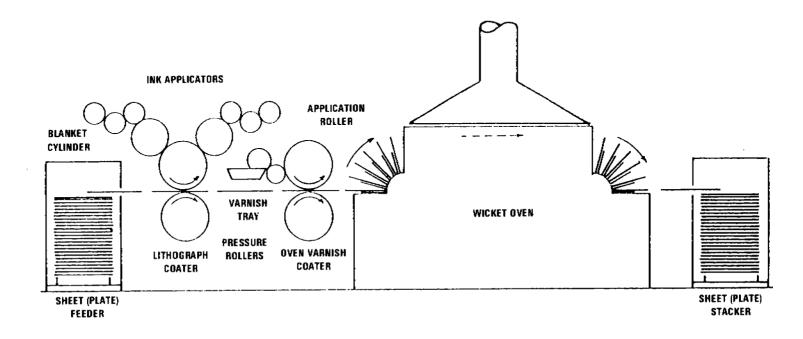
Figure 4.2.2.2-1. Three piece can sheet printing operation.<sup>7</sup>
