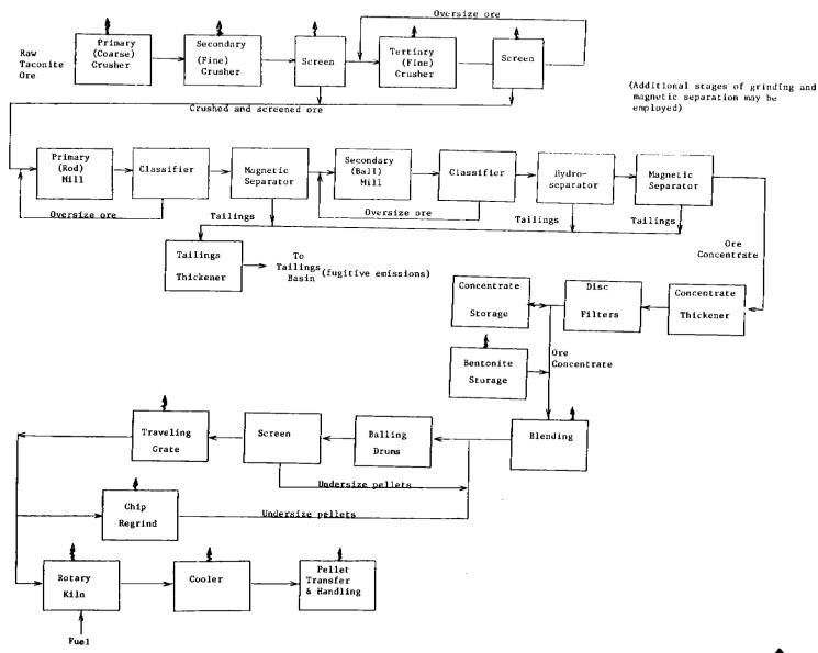
Figure 8.22-1. Taconite ore processing plant. (Process emissions are indicated by 7.)
