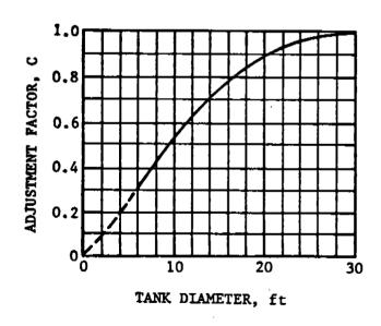
Figure 4.3-4. Adjustment factor (C) for small diameter tanks. $^2$
