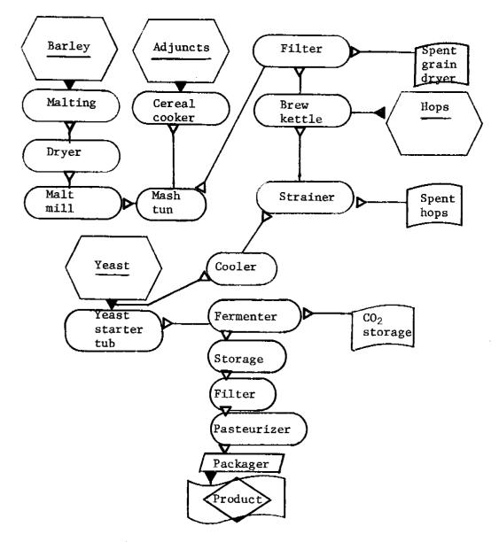
Figure 6.5.1-1. Flow diagram of a beer making process.
