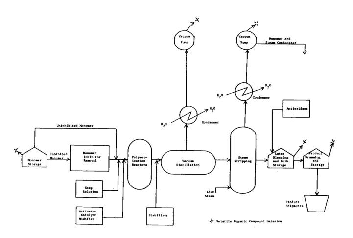
Figure 5.20-2. Typical process for latex production by emulsion polymerization.
