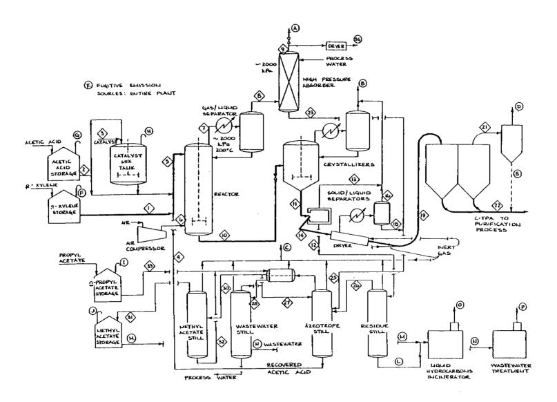
Figure 5.21-1. Crude Terephthalic Acid Process.
