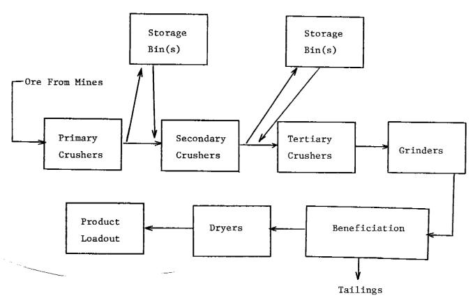
Figure 8.23-1. A metallic mineral processing plant.
