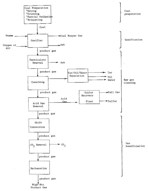
Figure 8.21-1. Flow diagram of typical coal gasification plant.
