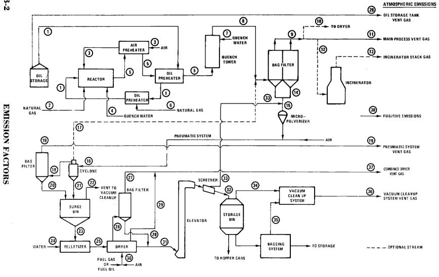
Figure 5.3-1. Flow diagram for the oil furnace carbon black process.
