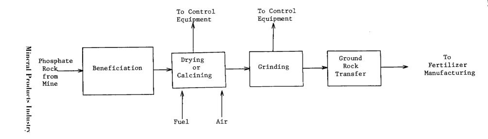
Figure 8.18-1. Typical flowsheet for processing phosphate rock.
