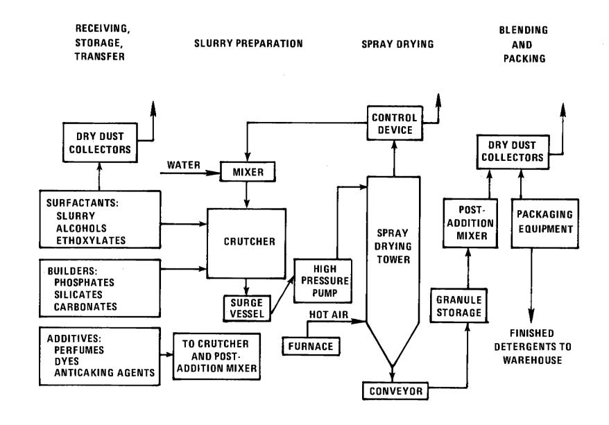
Figure 5.15-1. Manufacture of spray dried detergents.
