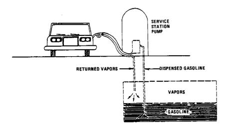
Figure 4.4-7. Automobile refueling vapor recovery system.
