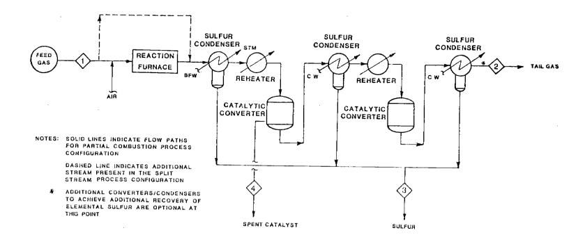
Figure 5.18-1. Typical flow diagram - Claus Process sulfur recovery.
