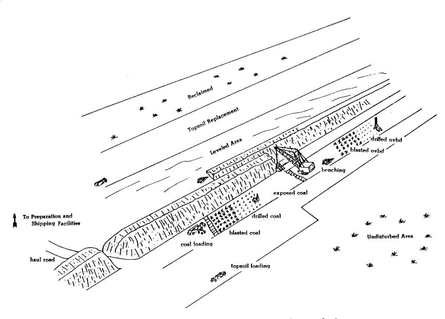
Figure 8.24-2. Operations at typical western surface coal mines.
