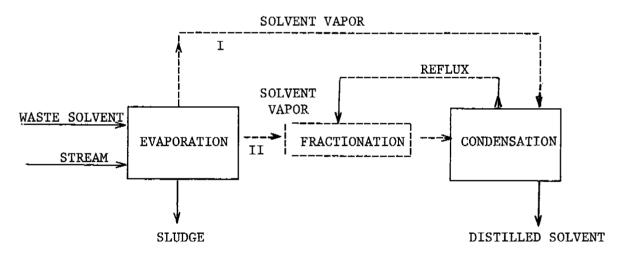
Figure 4.7-3. Distillation process for solvent reclaiming.
