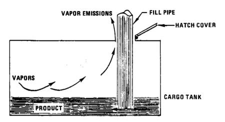
Figure 4.4-3. Submerged fill pipe.
