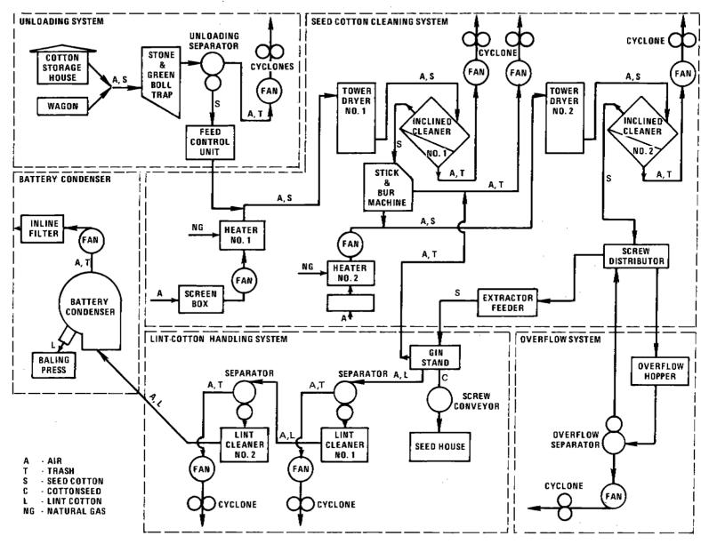
Figure 6.3-1. Flow diagram of cotton ginning process.<sup>2</sup>
