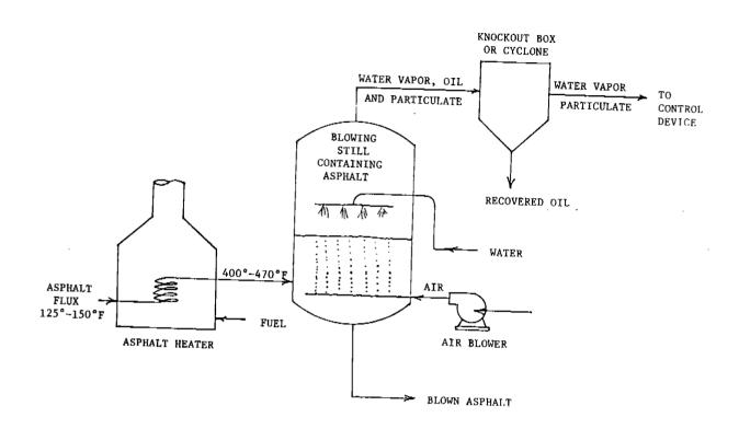
Figure 8.2.-1. Air blowing of asphalt.<sup>3</sup>
