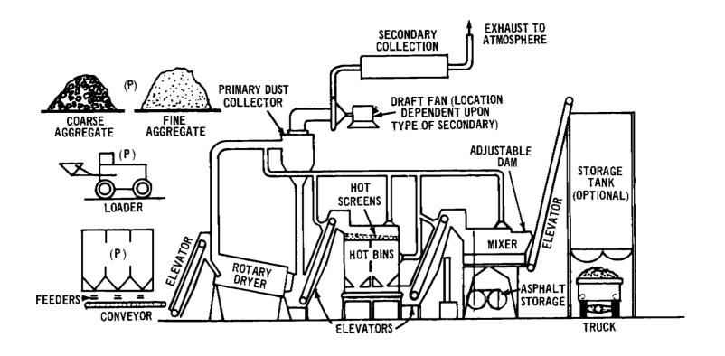
8.1 2. Continuous hot-mix asphalt plant. "P" denotes particulate emission points.1
