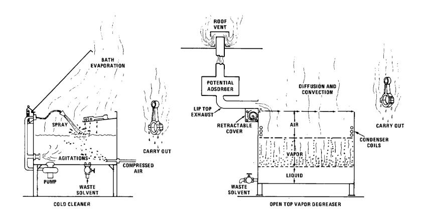
Figure 4.6-1. Degreaser emission points.
