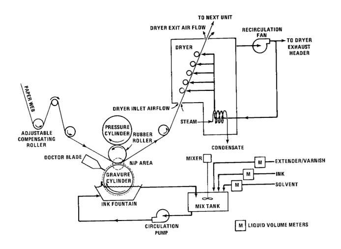
Figure 4.9.2-1. Diagram of a rotogravure printing unit.
