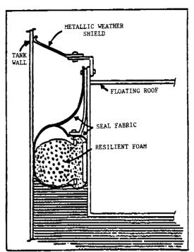
Liquid mounted seal with weather shield.
