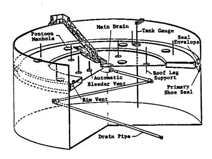
Figure 4.3-2. External floating roof tank. 1
