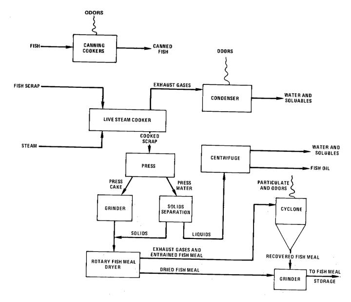
Figure 6.6-1. A generalized fish processing flow diagram.
