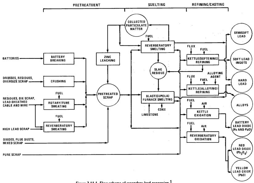
Figure 7.11-1. Flow scheme of secondary lead processing. 1
