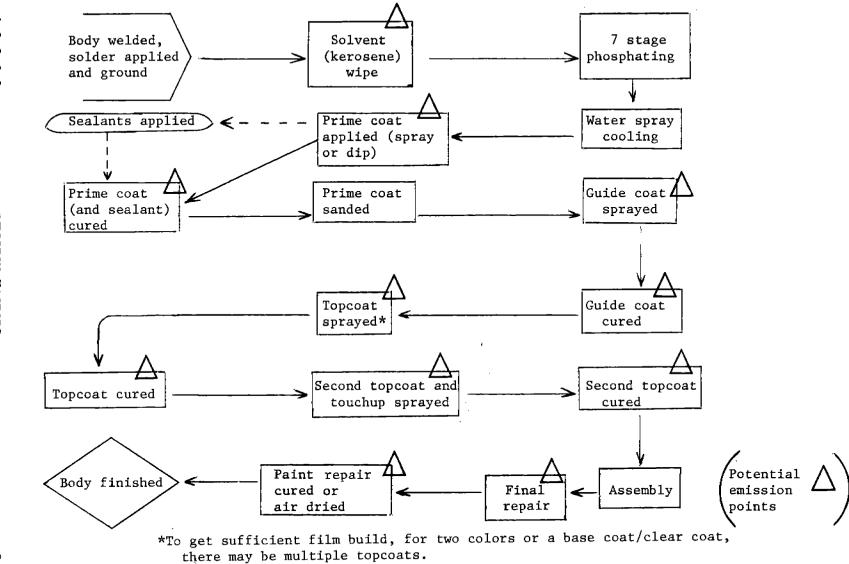
Figure 4.2.2.8-1. Typical automobile and light duty truck surface coating line.
