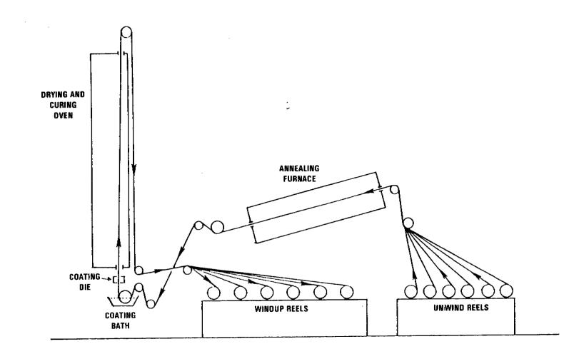
Figure 4.2.2.3-1. Wire coating line emission points.9
