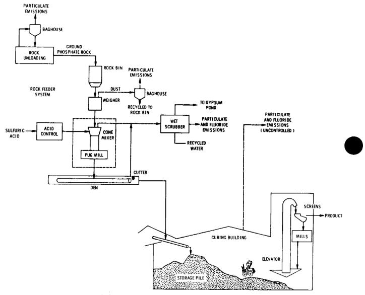
Figure 6.10.1-1. Normal superphosphate process flow diagram.
