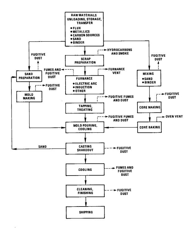
Figure 7.13-1. Typical flow diagram of a steel foundry.
