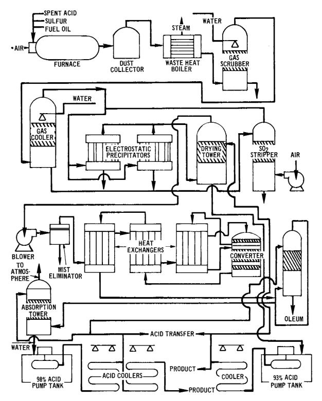
Figure 5.17-2. Basic flow diagram of contact process sulfuric acid plant burning spent acid.
