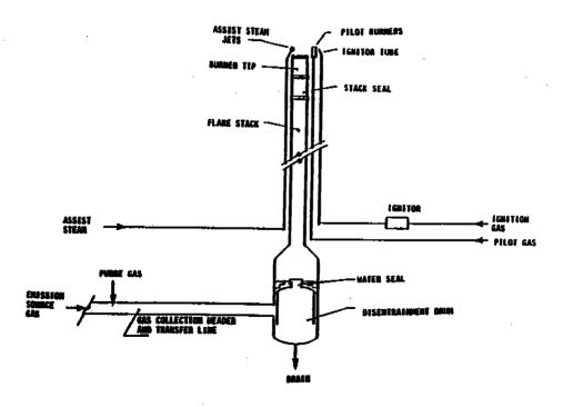
Figure 11.5-1. Diagram of a typical steam-assisted smokeless elevated flare.
