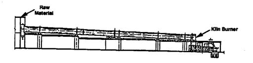
Figure 8.6-2. Conventional portland cement kiln.
