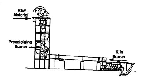
Figure 8.6-3. Typical portland cement preheater/precalciner.
