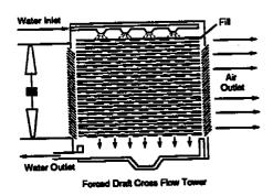
Figure 11.4-2. Mechanical draft cooling towers.
