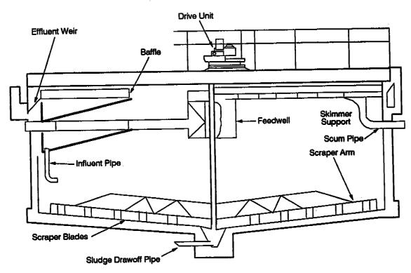
Figure 4.13-2. Example clarifier configuration.
