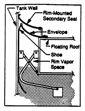
a. Shoe seal with rim-mounted secondary seal.
