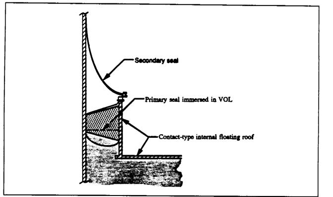
Figure 12.2-7. Rim-mounted secondary seal on an internal floating roof.<sup>5</sup>
