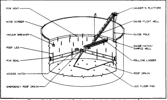
Figure 12.1-3. External floating roof tank (double-deck type).<sup>1</sup>
