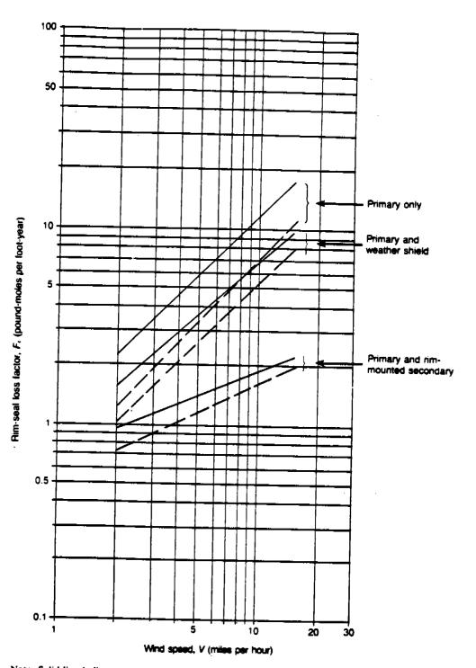
Note: Solid line indicates average-fitting seal; broken line indicates tight-fitting seal;  $F_r = K_r V^n$ .
