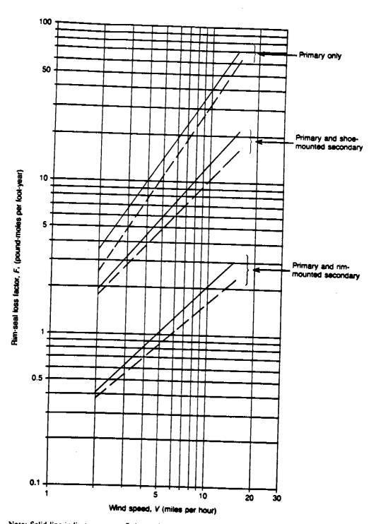
Note: Solid line indicates average-fitting seal; broken line indicates tight-fitting seal;  $F_i = K_i V^*$ .
