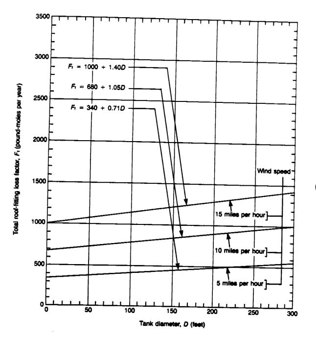
Figure 12.3-12. Total roof-fitting loss factor for typical fittings on pontoon floating roofs.<sup>3</sup>
