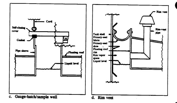
Figure 12.2-4. Roof fittings for external floating roof tanks.<sup>3</sup>
