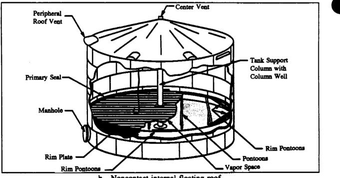
b. Noncontact internal floating roof.
