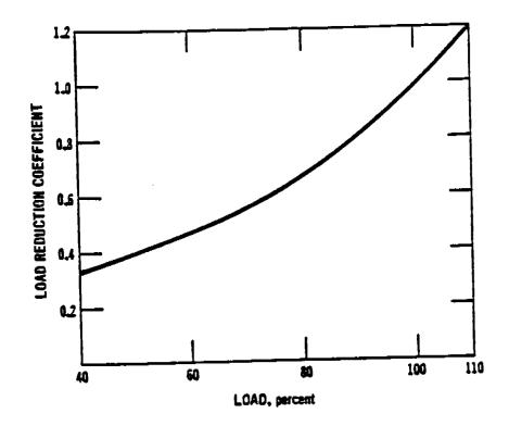
Figure 1.4-1. Load reduction coefficient as function of boiler load. (Used to determine  $NO_x$  reductions at recduced loads in large boilers).
