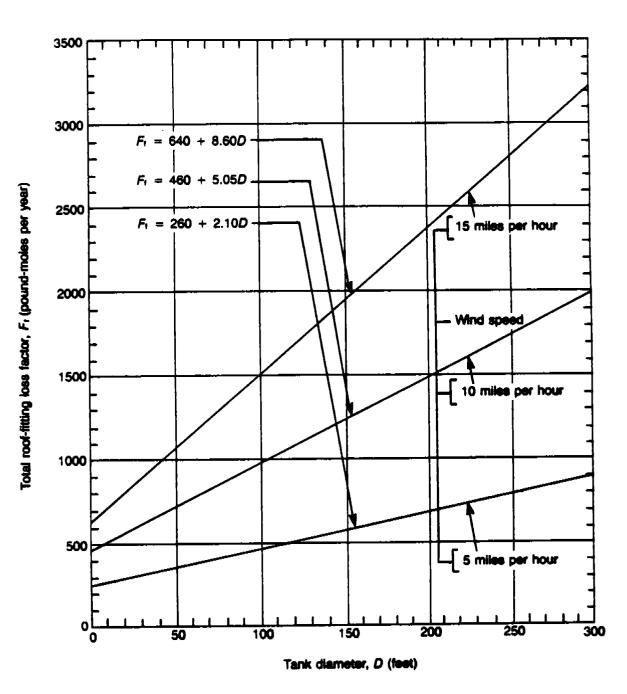
Figure 12.3-13. Total roof-fitting loss factor for typical fittings on double-deck floating roofs.<sup>3</sup>
