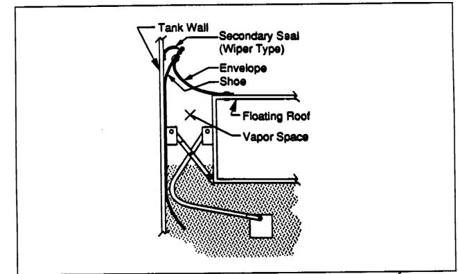
Figure 12.2-3. Metallic shoe seal with shoe-mounted secondary seal.<sup>5</sup>
