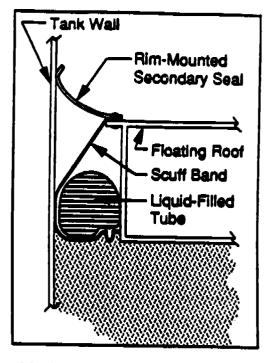
b. Liquid-filled seal with rimmounted secondary seal.
