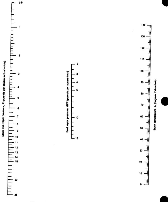
Figure 12.3-1A. True vapor pressure of crude oils with a Reid vapor pressure of 2 to 15 pounds per square inch.<sup>4</sup>
