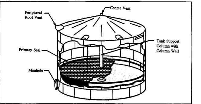
a. Contact internal floating roof
