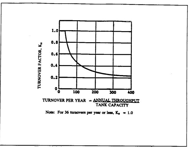
Figure 12.3-6. Turnover factor (K<sub>N</sub>) for fixed roof tanks.<sup>6</sup>
