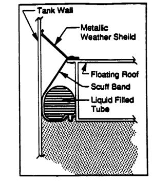
a. Liquid-filled seal with weather shield.
