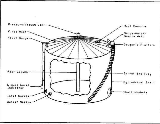
Figure 12.1-1. Typical fixed-roof tank.<sup>1</sup>
