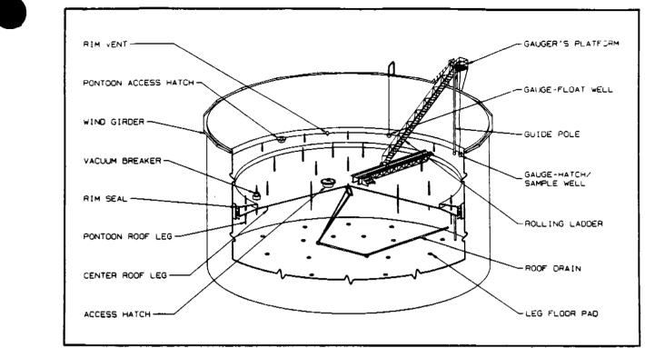
Figure 12.1-2. External floating roof tank (pontoon type).<sup>1</sup>
