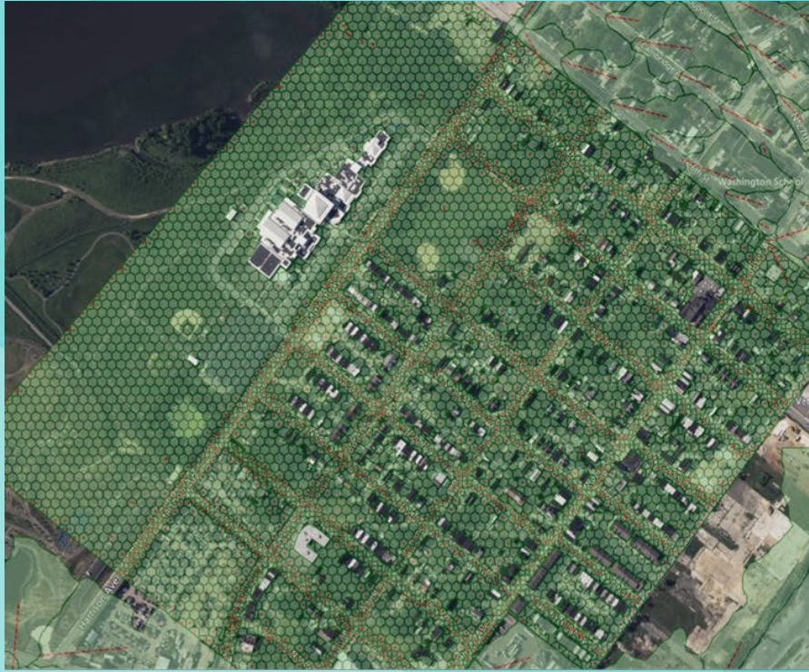
2D distributed subcatchments with buildings as obstacles
