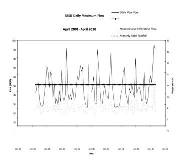
Figures 3 and 4 shows the Average Monthly Flows for the CRPCD and SESD, which exceed the nonexcessive infiltration standard for all but the driest months. This indicates that these systems experience high levels of groundwater infiltration into the system even during dry weather.
