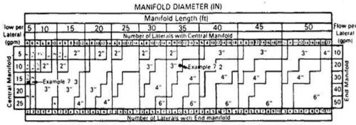
\*Computed for plastic pipe only. The Hazen Williams equation was used to compute headlosses through each segment (Hazen-Williams C = 150). The maximum manifold length for a given lateral discharge rate and spacing was defined as that length at which the difference between the heads at the distal and supply ends of the manifold exceeded 10 percent of the head at the distal end.
