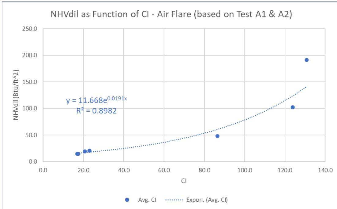
Figure 3. Example CI-NHV<sub>dil</sub> calibration for air assisted flares.
