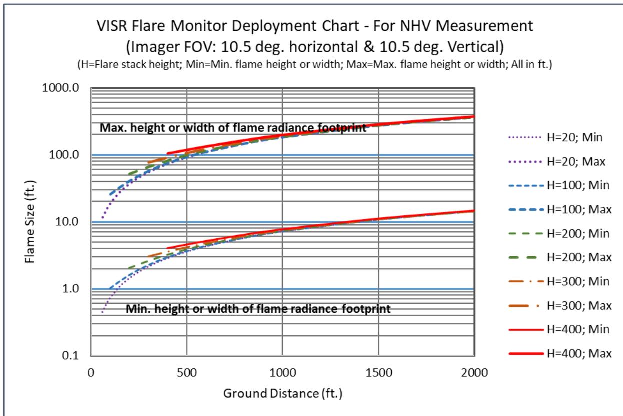
Note 1: The expected flame height or width is based on the thermal image footprint of the flame, and can be significantly larger than the flame footprint visible to naked eyes.
