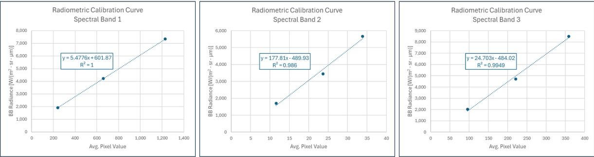
A Radiometric Calibration equation is derived from the calibration curve of each spectral band. Once calibration equations are established, the pixel readings of the VISR imager can be used to measure IR radiance in each spectral band.
