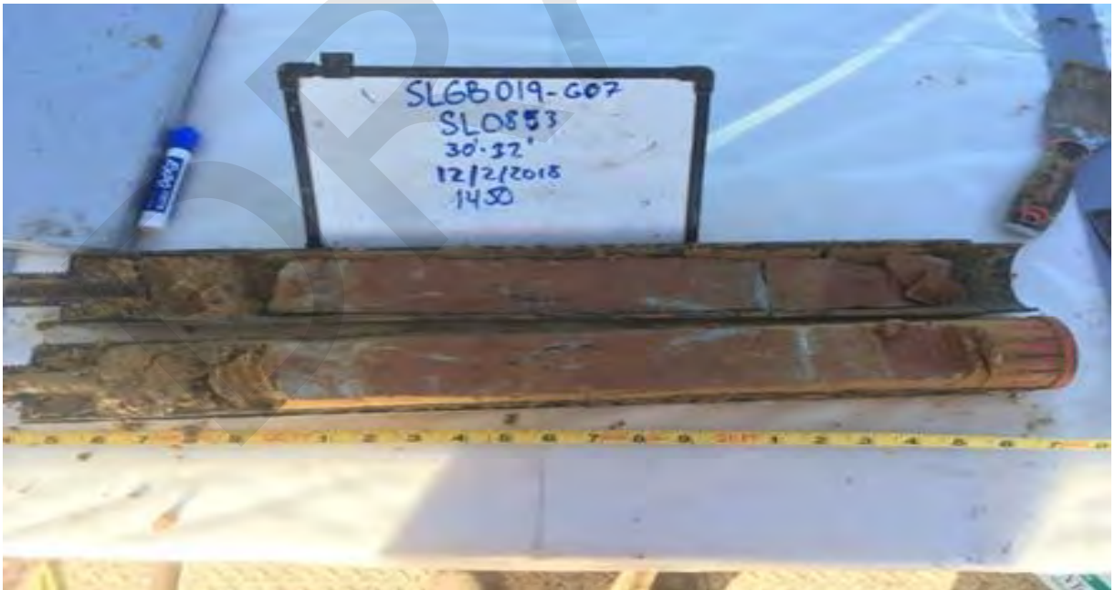
Photo 2 Figure D.2: Sample G07 (30 to 32 ft deep in borehole SLGB-019).
