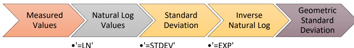
Figure 5-3. Process flowchart of the commands used in Excel to calculate the geometric standard deviation.
