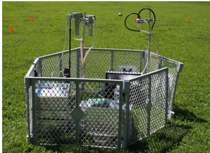
Figure 3-3. Typical field air sampling station setup (photo taken during pre-pilot testing), including particulate/metal, semivolatile organic compound (SVOC), active volatile organic compound (VOC), and passive VOC samplers. This configuration shows duplicate sample collection for each sample type.
