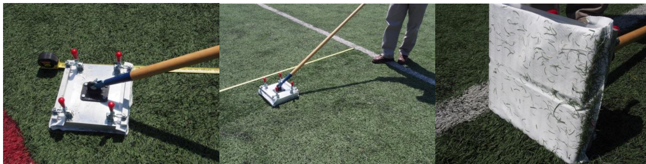
Figure 3. Wipe sampling push sled device with cotton dry wipe material attached.
