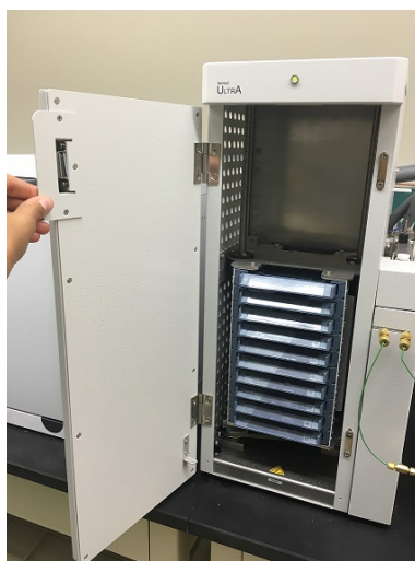
Figure 8. Opening the TD 50:50 door to access tube trays.
