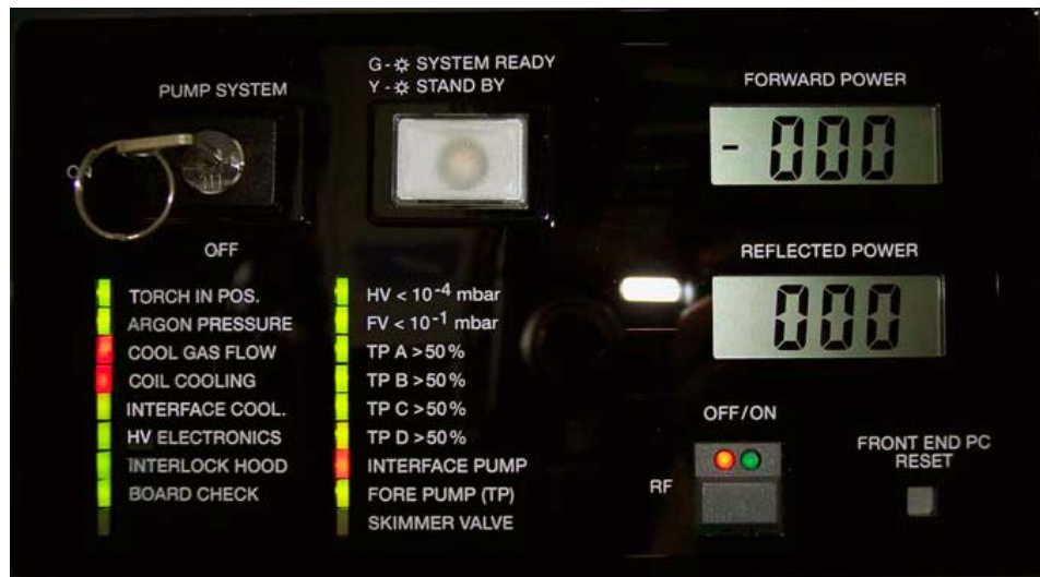
Figure 6. Status display panel when E2 is in standby.
