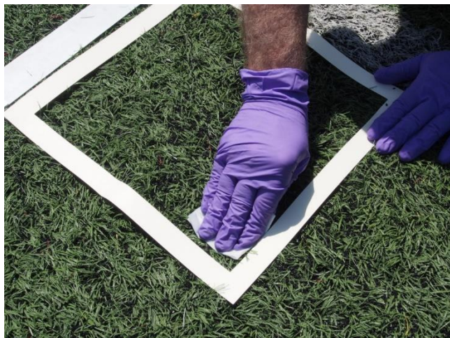
Figure 2. Wiping the turf surface in a S or Z-shaped pattern within the 929 cm 2 template area.
