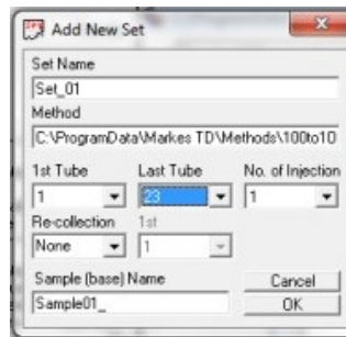
Figure 4. Selecting the number of tubes for analysis in the Add New Set dialog box.
