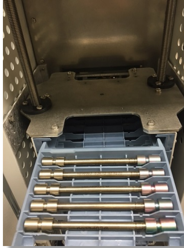
Figure 10. Loading the sample tray into the TD when full.
