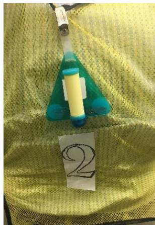
Figure 15. Radiello samplers deployed for personal monitoring (A) or stationary monitoring (B).
