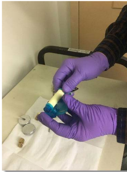
Figure 14. Screw the Radiello diffusive body onto the triangular support plate.
