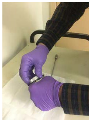
Figure 12. Remove end caps with Caplok tools.
