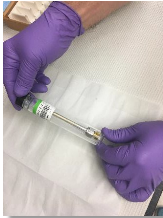
Figure 11A. Retrieve TD tube packed inside of glass vial from shipping container.
