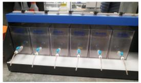
Bench- or pilot-scale testing of enhanced coagulation must be conducted by using representative water samples and adding 10 mg/L increments of alum (or equivalent amounts of ferric salt) until the pH is reduced to a level less than or equal to the enhanced coagulation Step 2 target pH shown in the following table:
