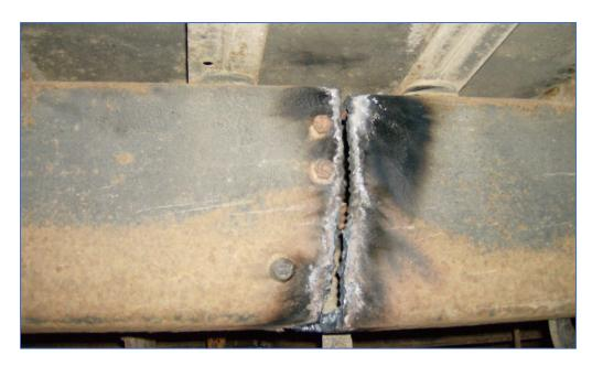
1) Chassis rail cut in half – DestroyedChassisRail[INSERT LAST 4 DIGITS OF VIN].jpg
