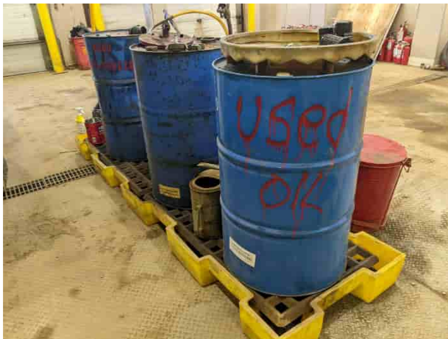
Photo No. 3 – Another view of the drum storage on a containment pallet within the garage portion of the building (HWMU-1). 22 June 2022
