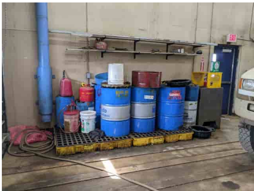
Photo No. 2 – Used glycol, oil, and petroleum, oil, and lubricants (POL) storage on containment on the west side of the garage bay of the HEMF building (HWMU-1). 21 June 2022
