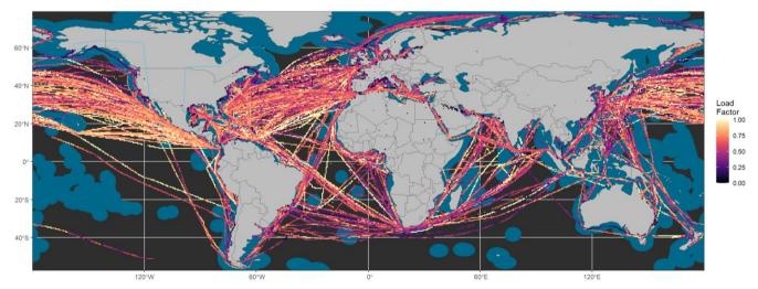
Figure 7: Map of median estimated engine load for sampled ships.
