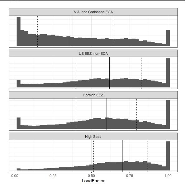
Figure 8: Histograms of estimated ship engine load factors for ships operating in different geographic regions.
