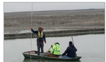
Compliance Advisors conducting a solids inventory at a lagoon in Wyoming. Photo credit: ERG
