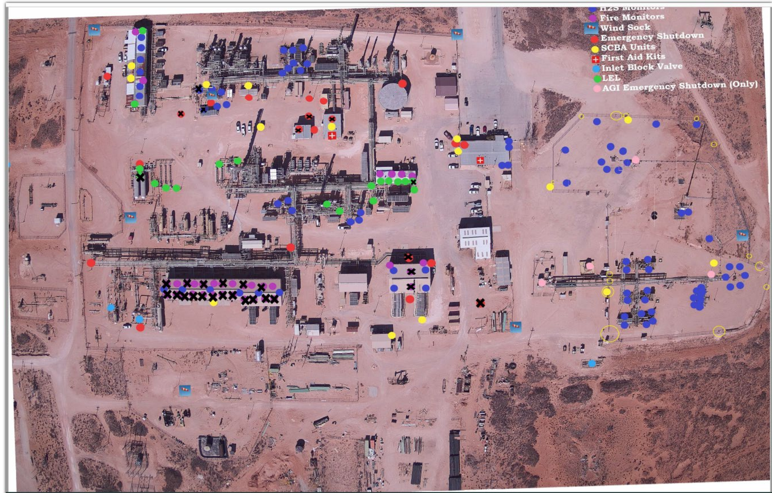
Figure 37-3: Location of alarms, monitors, and safety equipment at the Maljamar Gas Plant and Maljamar wells. The blue circles are the H 2 S monitors.
