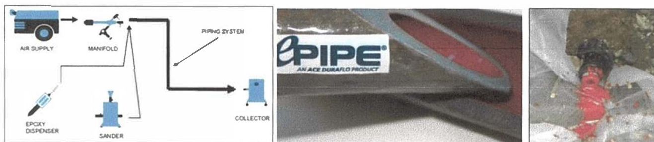
Figure 4. A schematic of the ePipe epoxy application process; promotional photo of an epoxy coated lead pipe; and field photo of excess epoxy being blown from lead pipe in demonstration installation in Providence, RI.
