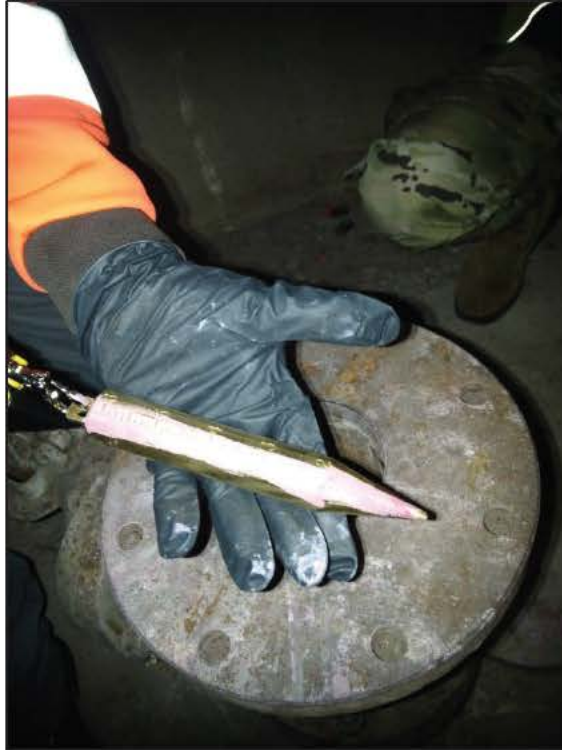
Figure 26 - Plumb bob after retrieval in gauging Tank 20. Fuel paste that changes color in contact with fuel indicated that (b) (3) (A) of fuel present at location where bob struck tank bottom (EPA Inspection Photo Log).
