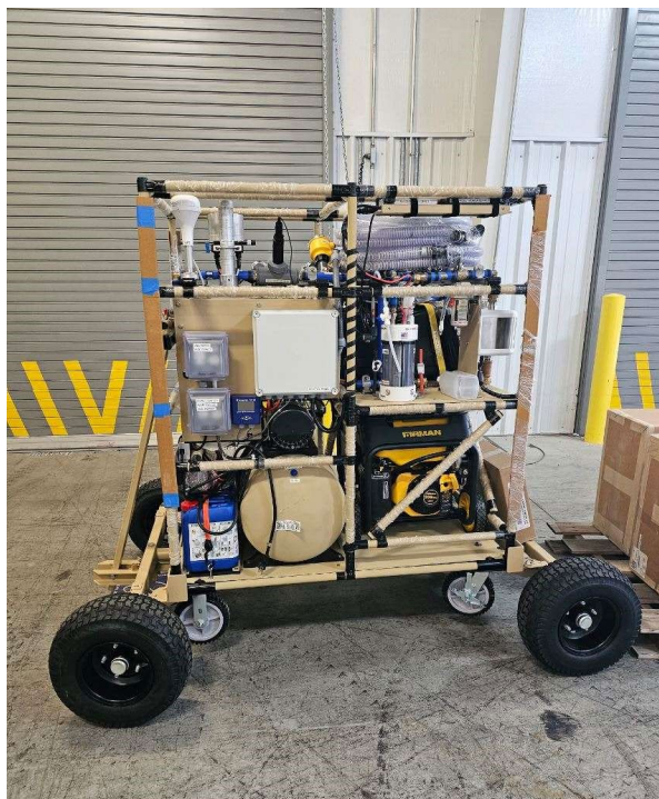
The DRIPS with GPS, remote telemetry, chemical resistant coating, and all-terrain wheels.
