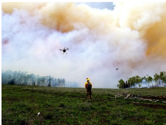
sUAS-based emission sampling during stand replacement burns in Fishlake National Forest, Utah. Jess Juchtzer, Desert Research Institute, used by permission.
