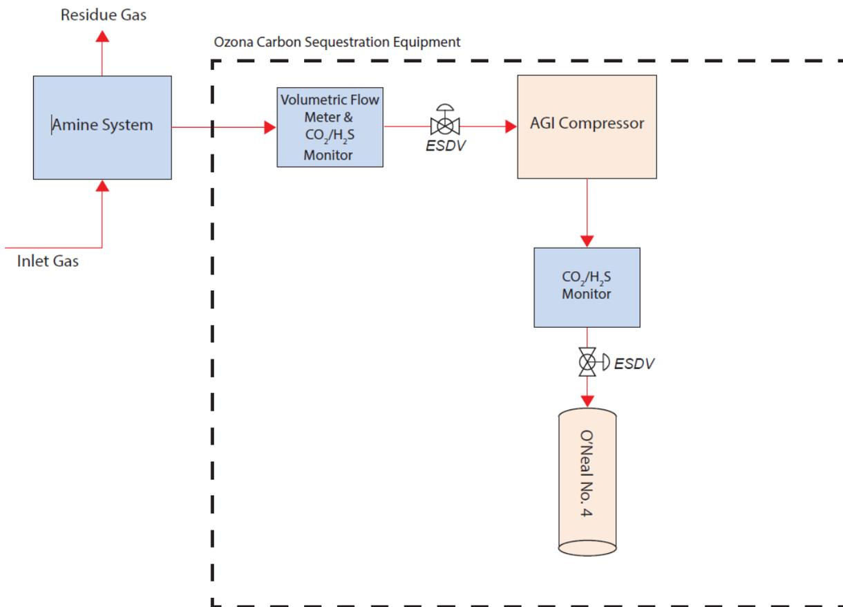
Figure 37 – O’Neal No. 4 Process Flow Diagram
