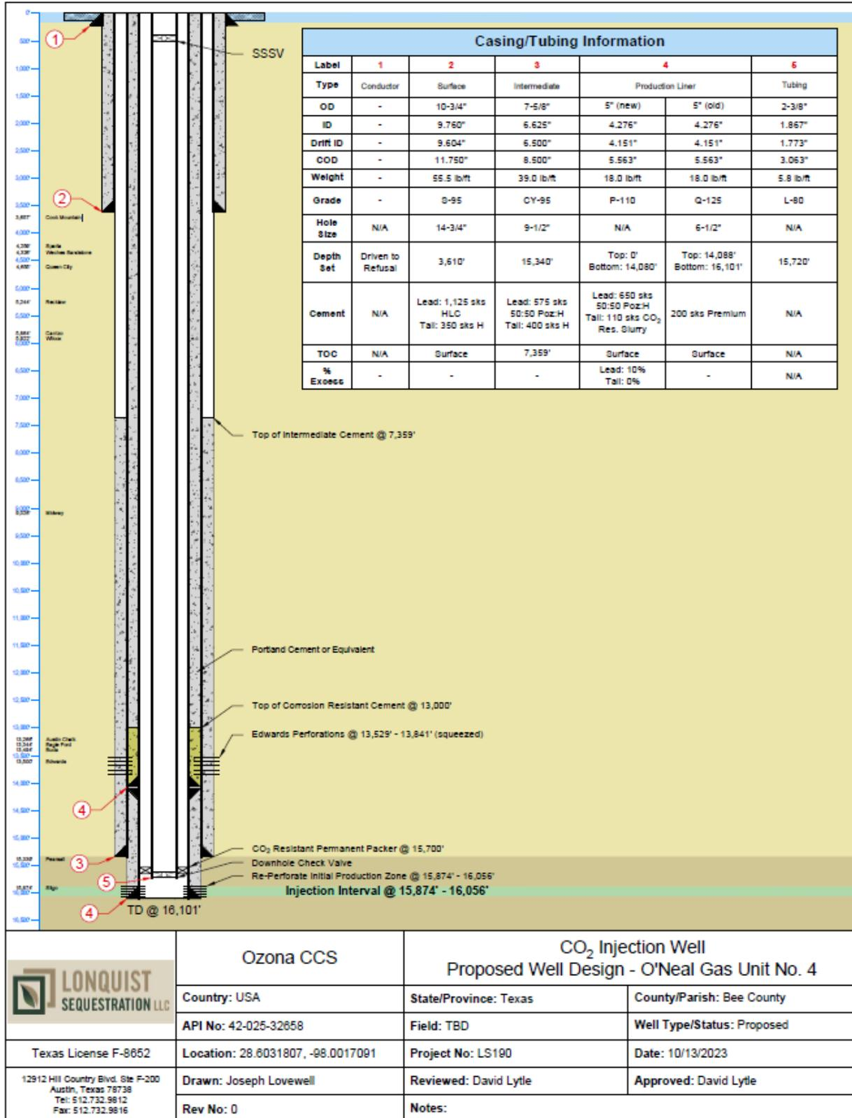
Figure 32 – O’Neal No. 4 Wellbore Schematic
