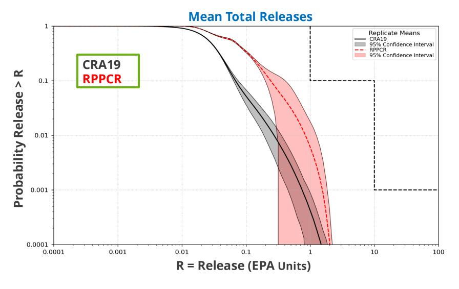
The WIPP facility as modeled in the RPPCR PA remains in compliance with EPA containment requirements.
