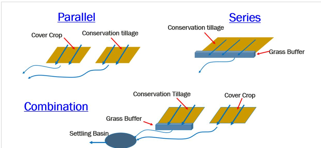
Figure A-1. Illustration of BMPs in parallel and series configurations and a combination of both.
