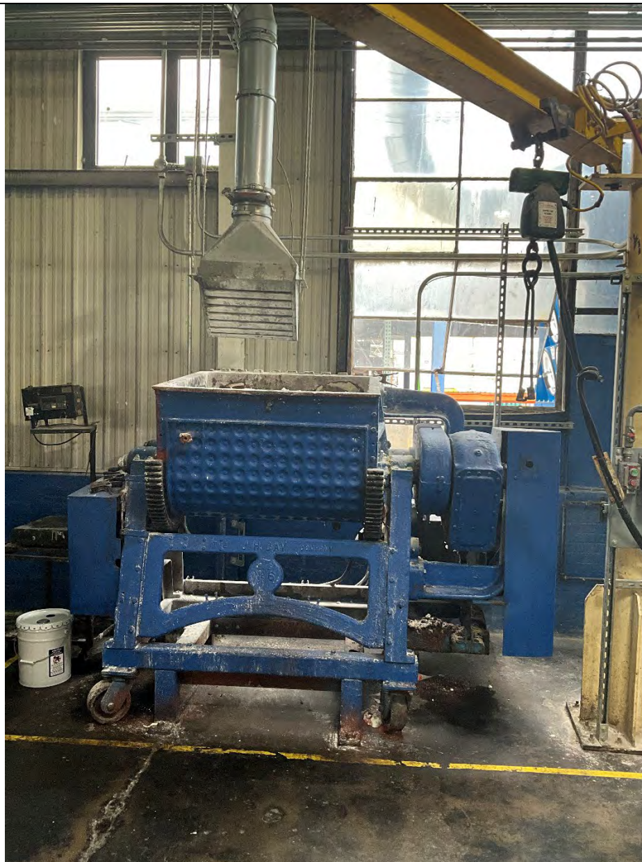
Dough mixer, which was empty and the associated emission collection system (facing Northeast)
