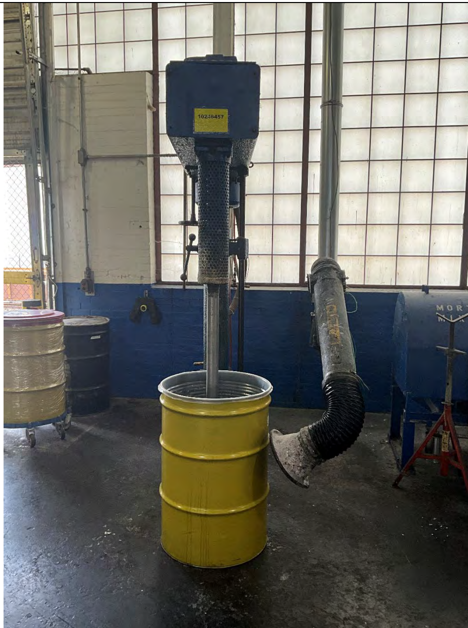
45-1 mixer, which was empty and its associated emission collection system (facing Southwest)
