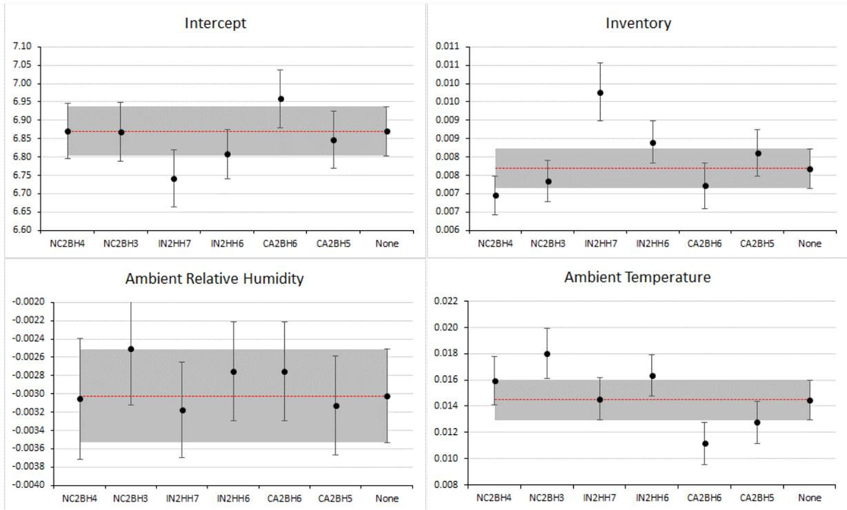
**Figure 6-3. Comparison of variation in coefficients and standard errors for PM<sub>10</sub> high rise house model.**
