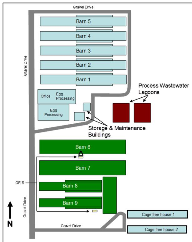
**Figure 8-19. Overhead view of IN2H/IN2B, with the PM inlet measurement location indicated by a triangle. (Ni et al. 2010a).**
