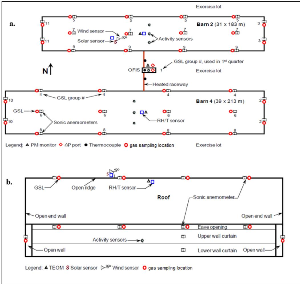
Figure 8-21. Overhead (a.) and side (b.) view of sensor measurements at WA5A barn (Ramirez-Dorrnsoro et al. 2010).
