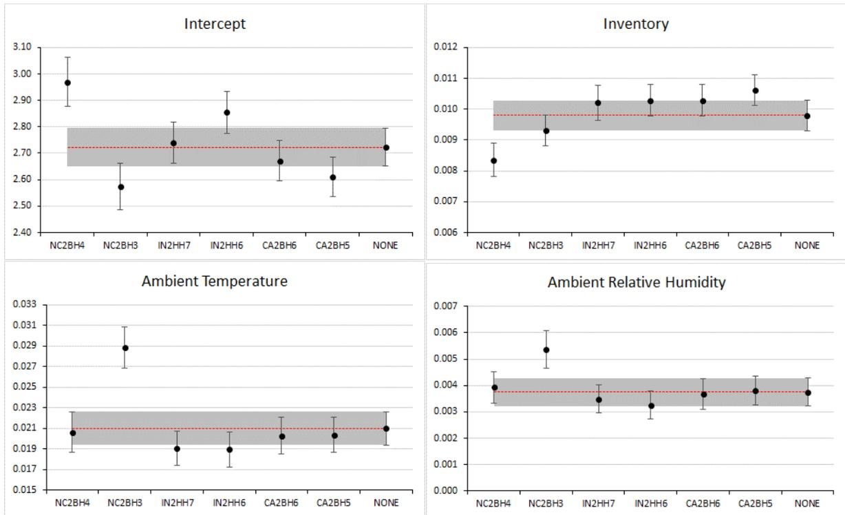
**Figure 6-2. Comparison of variation in coefficients and standard errors for H<sub>2</sub>S high rise house model.**
