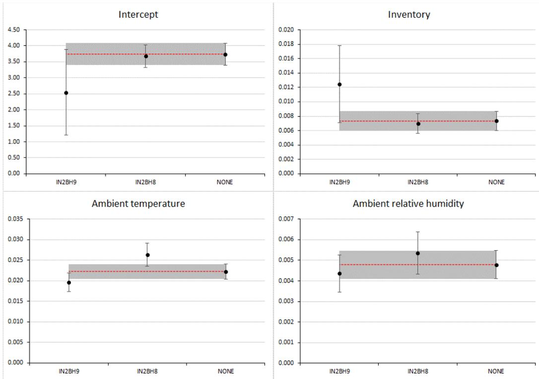
**Figure 6-7. Comparison of variation in coefficients and standard errors for H<sub>2</sub>S manure belt house model.**
