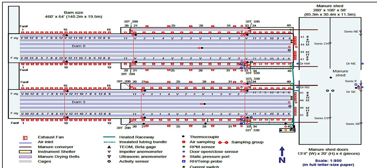
Figure 8-22. Overhead view of sensor measurements at IN2B (Ni et al. 2010b).
