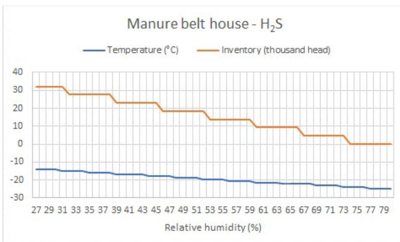
Figure 8-12. Maximum values at which the manure belt house models yield negative emissions. Visualization of the results for H<sub>2</sub>S.
