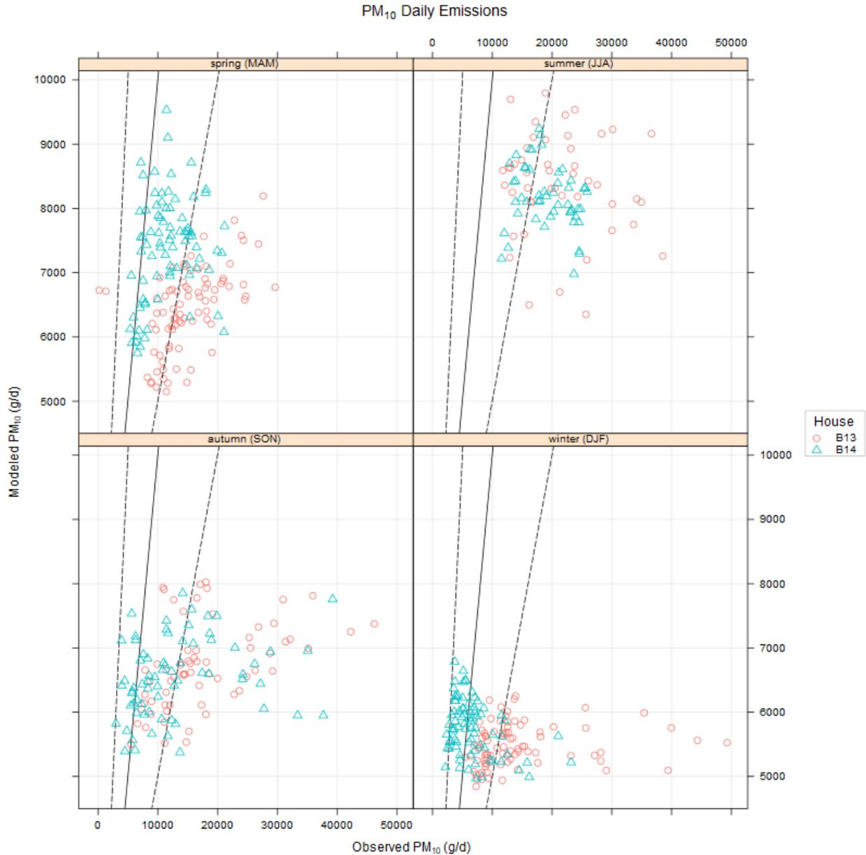
**Figure 8-18. Scatter plot of the observed PM<sub>10</sub> emissions at the APECAB IN high rise site versus the emissions model estimates.**
