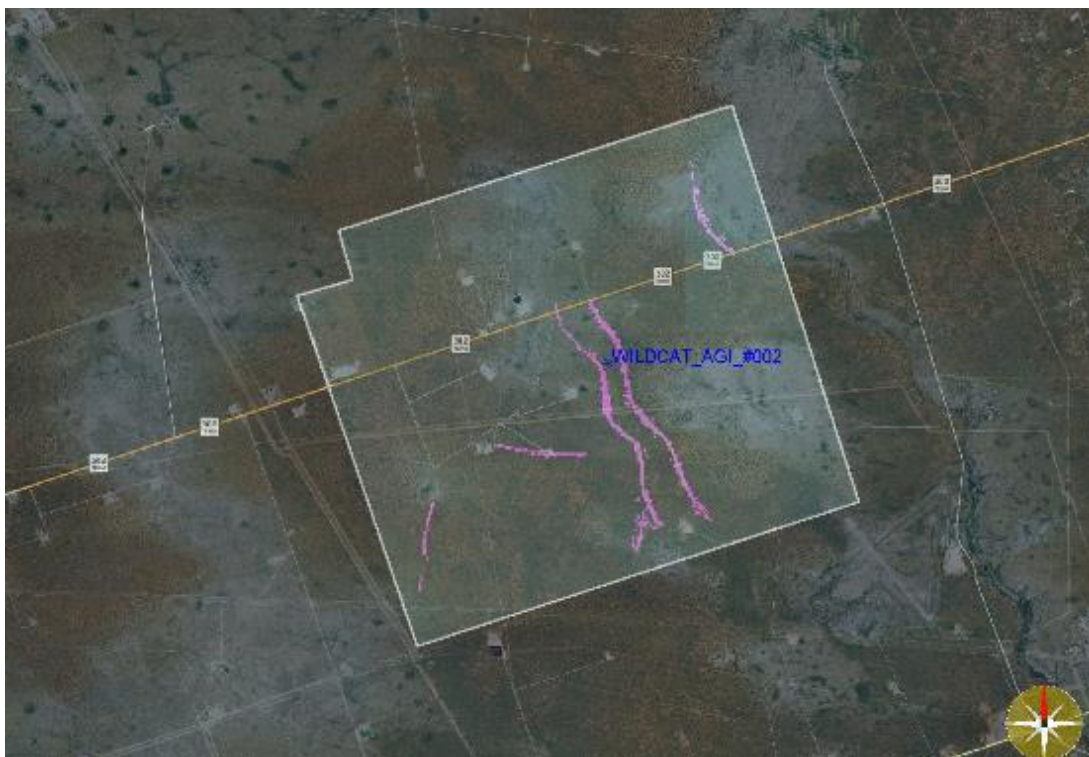
Figure 3.8.2: Map view of the simulation model of the Wildcat AGI #1 and #2 wells. Six (6) potential major faults (pink color), passing through the lower injection interval, were identified by 3D seismic analysis.
