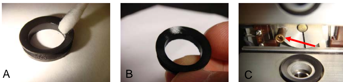
Figure 10-11. Photographs illustrating application of silicone grease to the V-seals and O-rings (Panels A, B) and repositioning of the brass bushing on the motor cam post (Panel C, arrow).
