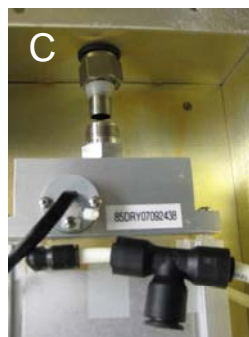
Figure 10-19. Photographs illustrating the Swagelok fittings at the top and bottom of the dryer that must be loosened so the inlet may be raised to allow dryer removal.
