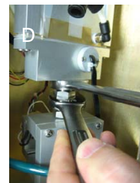
Figure 10-19. Photographs illustrating the Swagelok fittings at the top and bottom of the dryer that must be loosened so the inlet may be raised to allow dryer removal.
