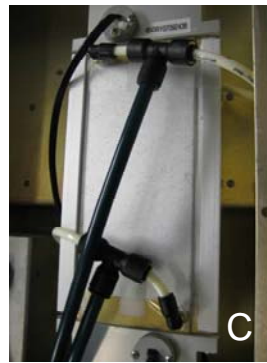
Figure 10-18. Photographs illustrating plumbing disconnections needed to facilitate dryer removal.
