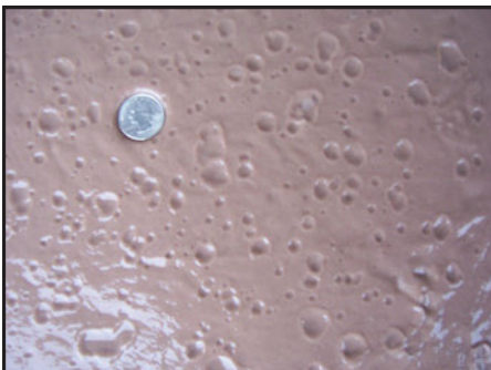
Properly Thickened Base Mix (Quarter used for perspective)
