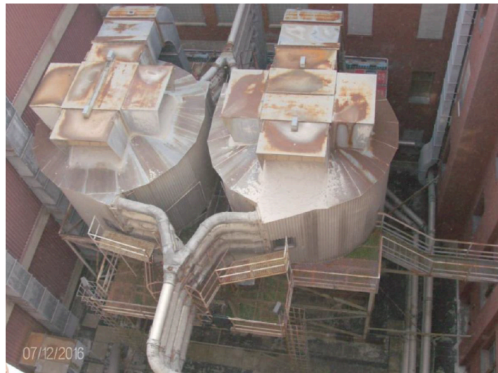
View of two cyclone dust removal units attached to paper baling equipment
