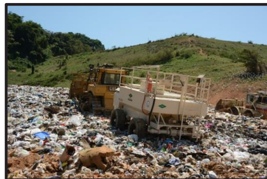
Proper orientation of equipment on slope
