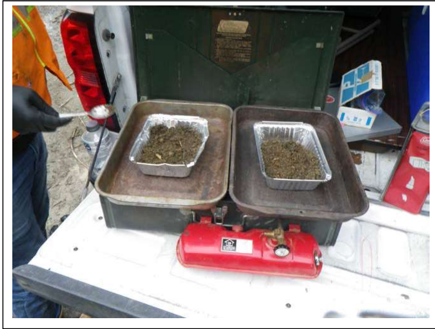
Photo 3: Drying the sub-portion sampling prior to sieving.
