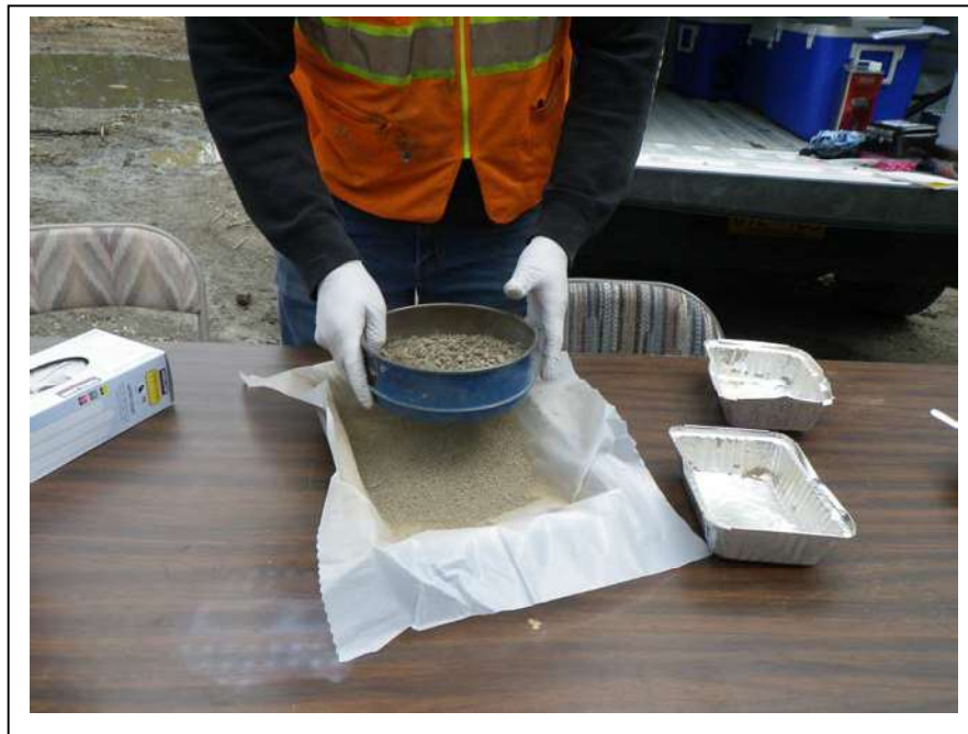
Photo 4: Hand sieving sub-portion through a #10 (2mm) sieve.
