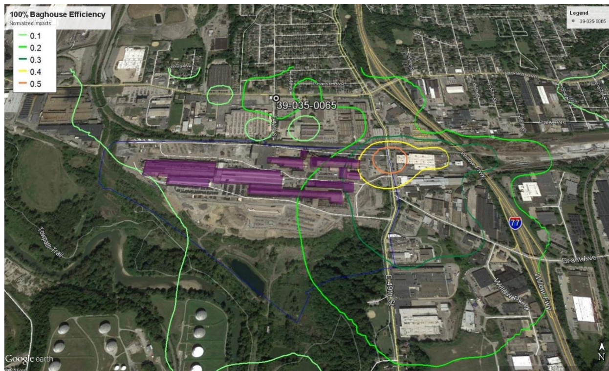
Figure 18: Isopleths of SO2 concentration when 100% of emissions from Charter Steel are emitted from the baghouse stacks
