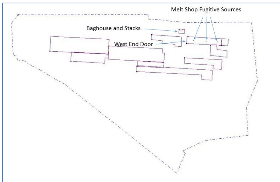
Figure 15: Layout of buildings and sources at the Charter Steel Facility
