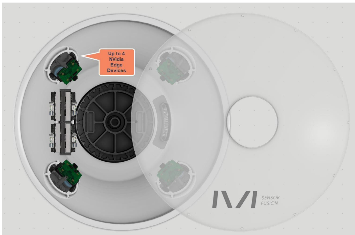
Figure 6.2. Internal view of the Minerva Platform showing the location of up to 4 edge computing devices.
