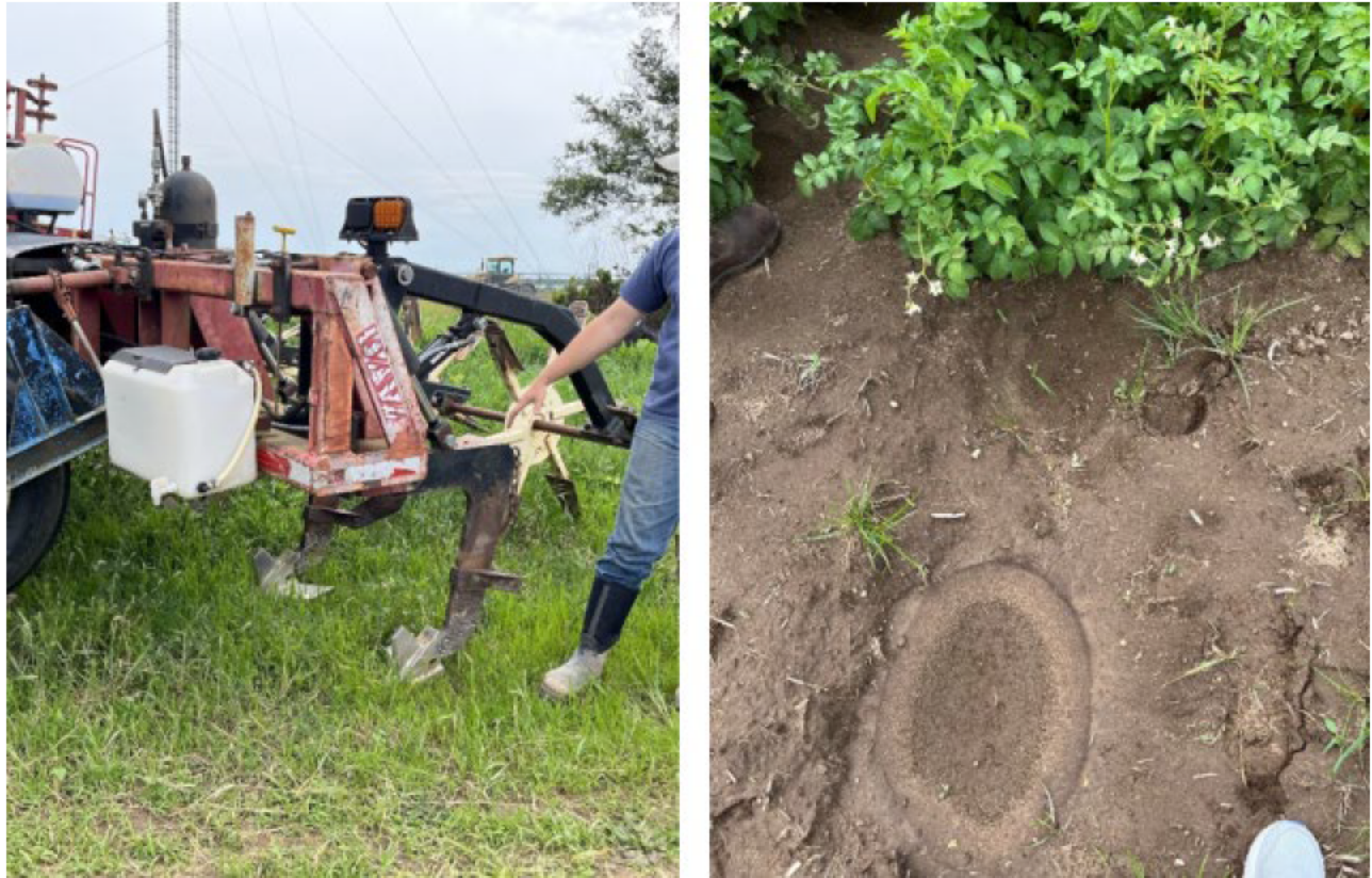
Figure 4. Reservoir tillage equipment creates depressions in a potato field that collect rainfall or irrigation water and later provide soil moisture for the crop. Photos by Rebecca Waterworth.
