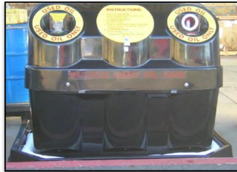
From left: Used oil containers on top of a secondary containment pallet; a used oil collection tank surrounded by spill containment.
