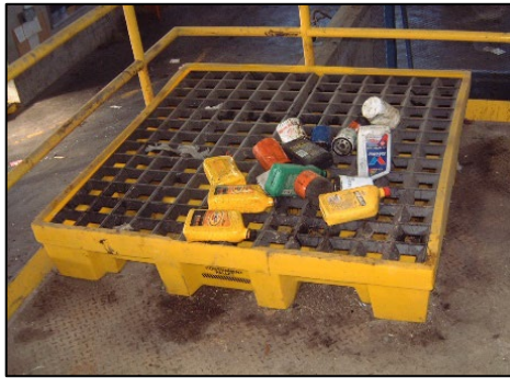
From left: Used oil containers on top of a secondary containment pallet; a used oil collection tank surrounded by spill containment.
