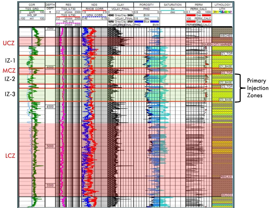
**Figure 9. Petrophysical log of the Nueces Minerals No. 1 well with the Queen City Formation primary injection interval annotated on the right and the individual injection and confining zones annotated on the left. The injection interval is comprised of Injection Zone 2 (IZ-2) and Injection Zone 3 (IZ-3). Injection Zone 1 (IZ-1) was mapped but not included as part of the CO<sub>2</sub> plume model.**
