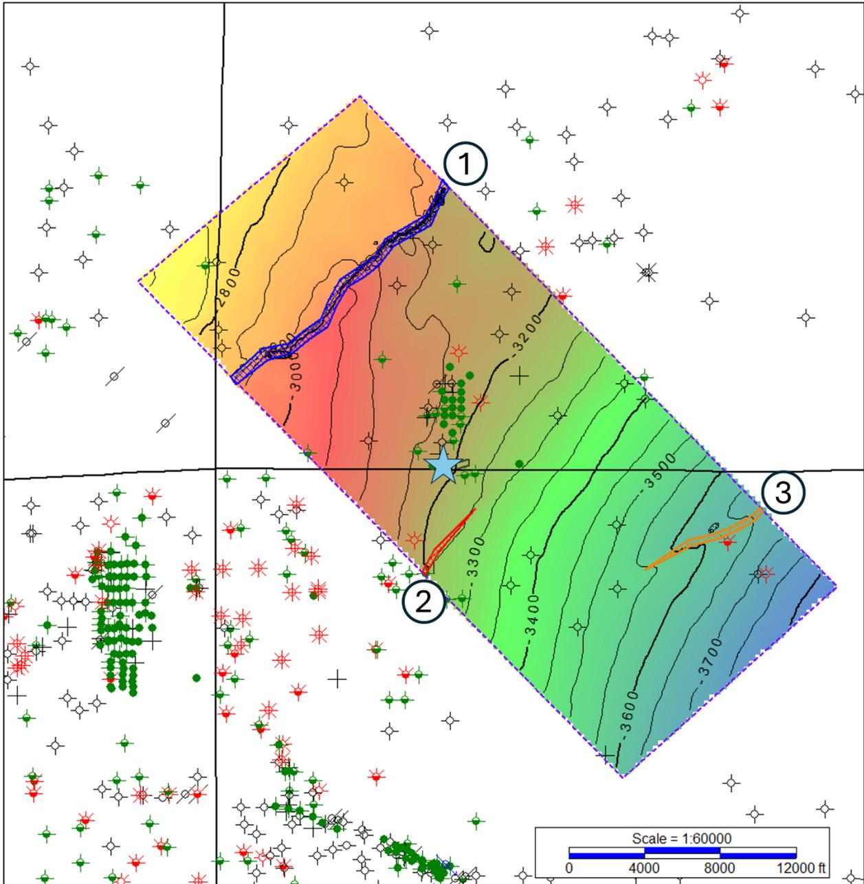
**Figure 7. Top Queen City Formation structure in feet TVDSS with a contour interval of 50 feet. The injection well is highlighted with the blue star and all existing oil and gas wells are shown. Faults are indicated by the colored polygons and numbers. North is up.**
