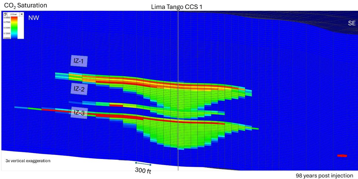
**Figure 23. Northwest to southeast cross section depicting the CO<sub>2</sub> saturation profile of the model for the injection from Lima Tango CCS 1 after 12 years of injection (upper) and after 98 years after injection stops (lower). Color scale at the upper left indicates CO<sub>2</sub> gas saturation. Queen City injection zones are annotated. Injection was only modeled for IZ-2 and IZ-3. Cross section location is shown on Figure 18.**
