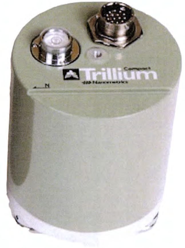
3-component ground motion sensor (vertical, north-south, east-west)
