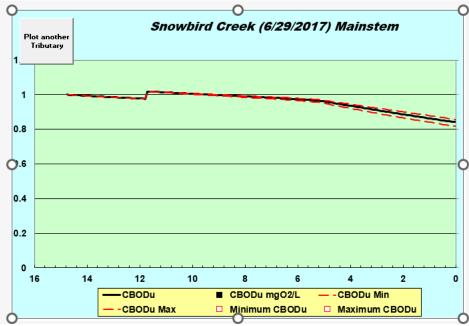
2. QUAL2K results graph for CBOD. Shows that the addition of effluent to Snowbird Creek does not cause CBOD to vary from upstream CBOD in a significant way
