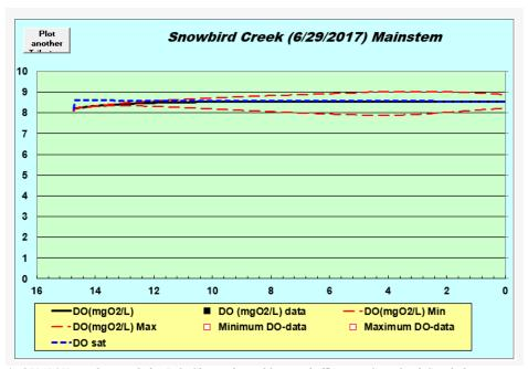
1. QUAL2K results graph for DO. Shows that addition of effluent to Snowbird Creek does not cause DO to vary from DO saturation in a significant way
